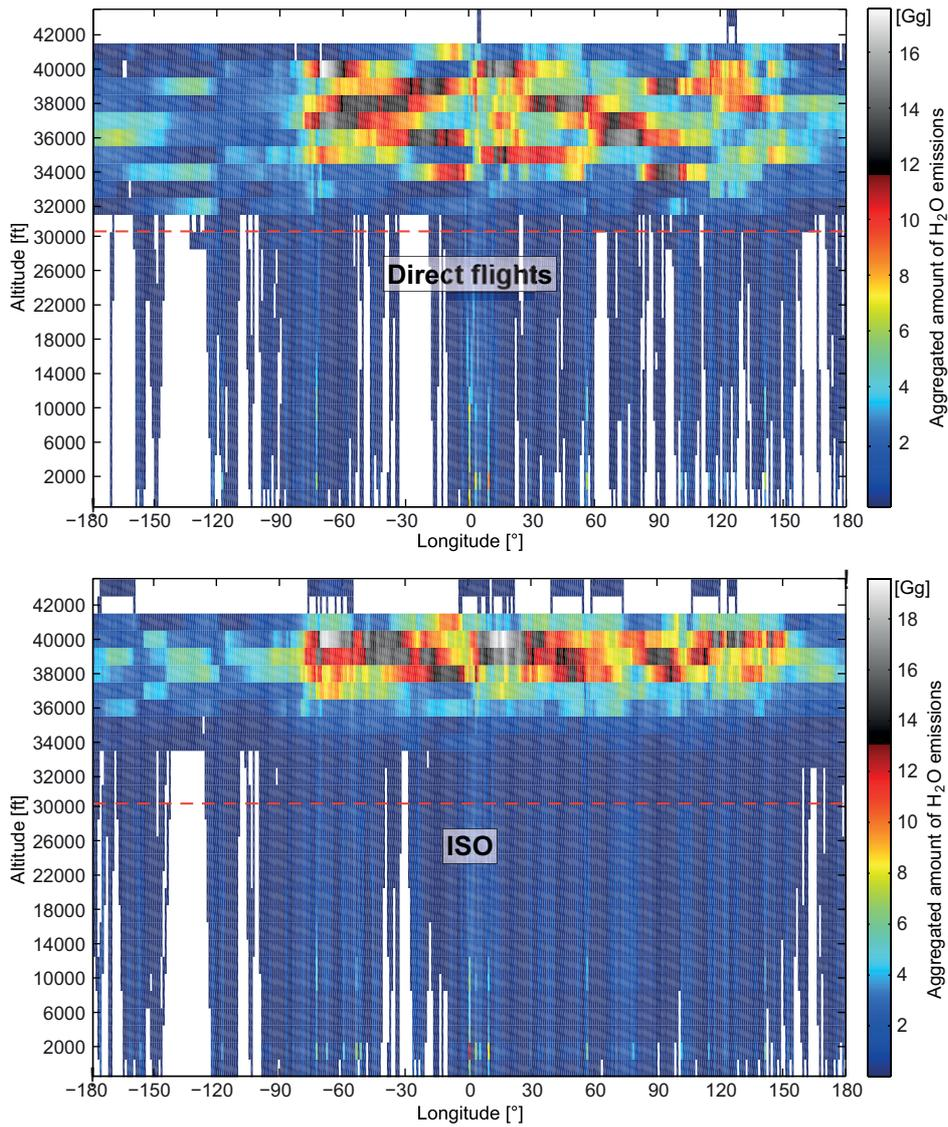
**Figure 6:** Distributions of H<sub>2</sub>O emissions (absolute values meridionally aggregated) in longitude-altitude plane for the direct flight mode (top) and the ISO mode (bottom); red line depicts a break in the vertical scale.
