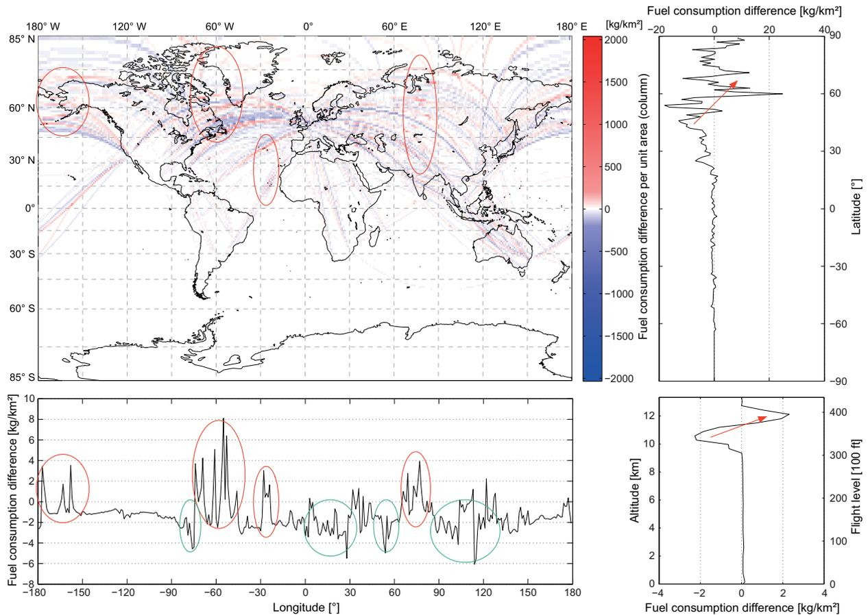
**Figure 4:** Redistribution of global fuel consumption due to ISO on long-haul missions (differences from direct flight scenario) in the first quarter of 2010; top left: geographical distribution of changes in the fuel sums per grid column; top right: latitude profile (zonal); bottom left: longitude profile (meridional); bottom right: altitude profile.
