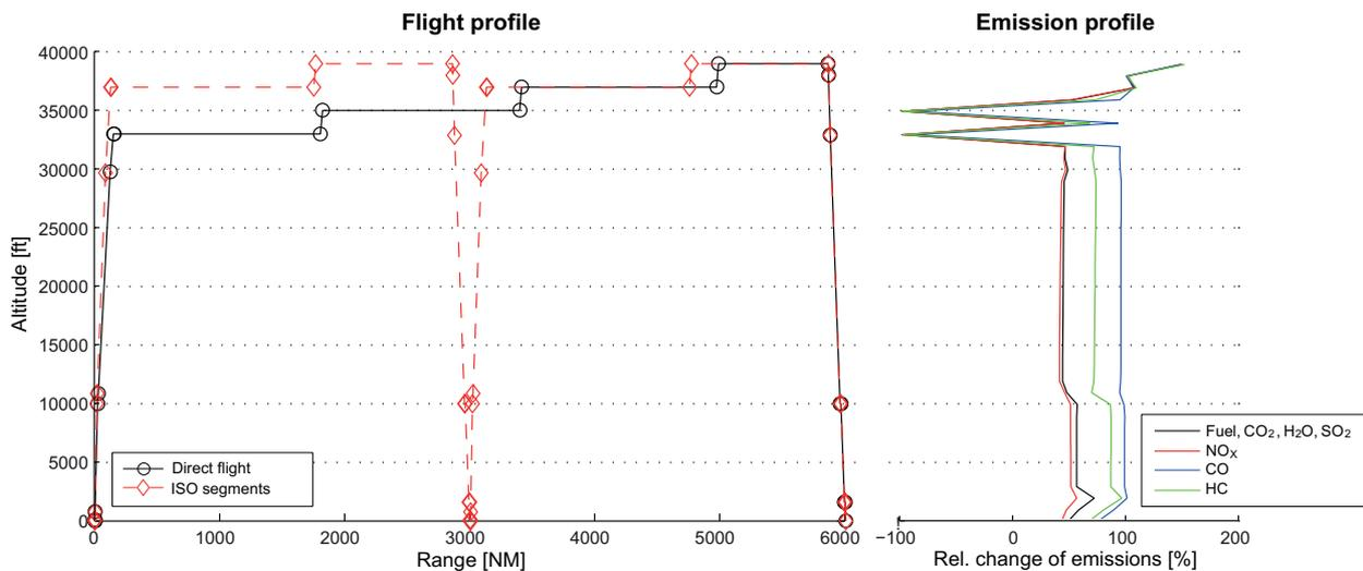
**Figure 2:** Change of flight altitudes and vertical emission distribution due to ISO shown on an exemplary 6000 NM mission flown with an Airbus A340-600 aircraft assuming an ideal intermediate landing (in the middle).
