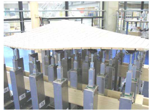
Fig. 3: prototype of a flexible mould built by Rietbergen and Vollers
