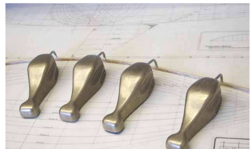
Fig. 5: Splines used e.g. for ship design
