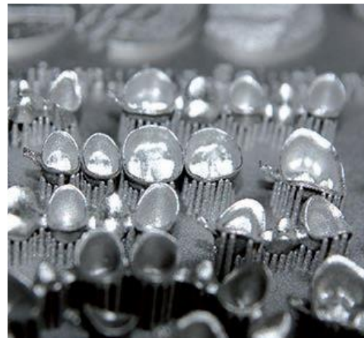
Figure H-1 A building platform can be charged with up to 450 crowns (EOS, 2013a)
