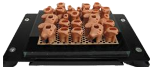
Figure H-2 3D printed hearing aid outer shells (Peels, 2011).
