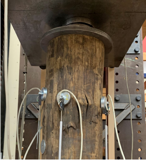
Figure 14: Failure in compression around knots
