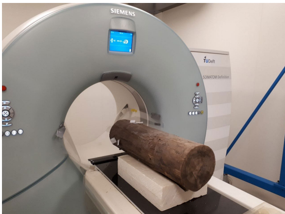
Figure 9: CT scanning test of retrieved timber pile
