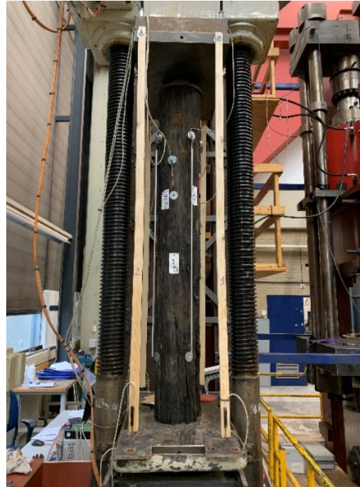
Figure 12: Large scale compression test set-up.
