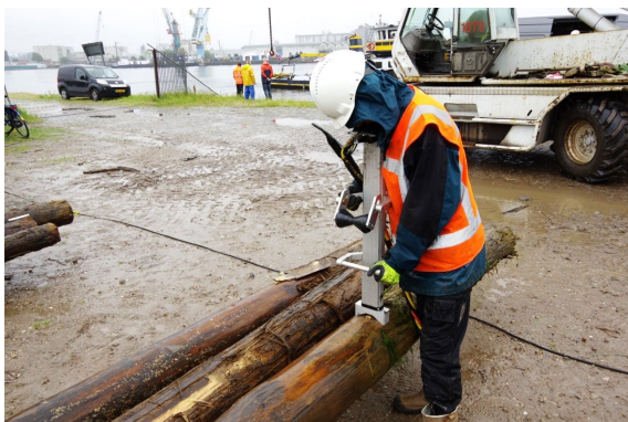
Figure 6: Microdrill in use on an excavated pile.
