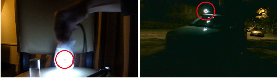
Figure 2.2: Our tracking algorithm automatically finds the center of the light sources with different sizes, occlusions and reflections.
