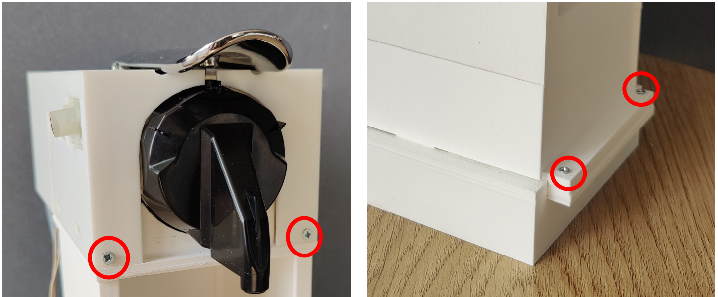
Figure 78: Screws visible when the coffee machine is assembled
