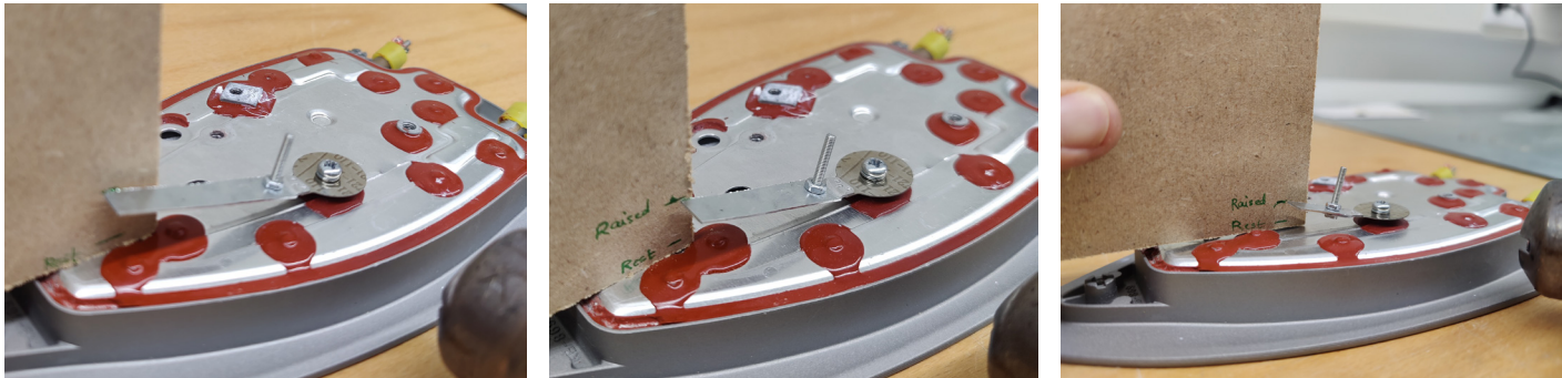
Figure 137: Deflection of the bimetal at different lengths
