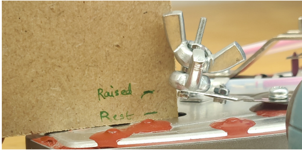
Figure 71: The bimetal carrying 15 gram of weight at its tip
