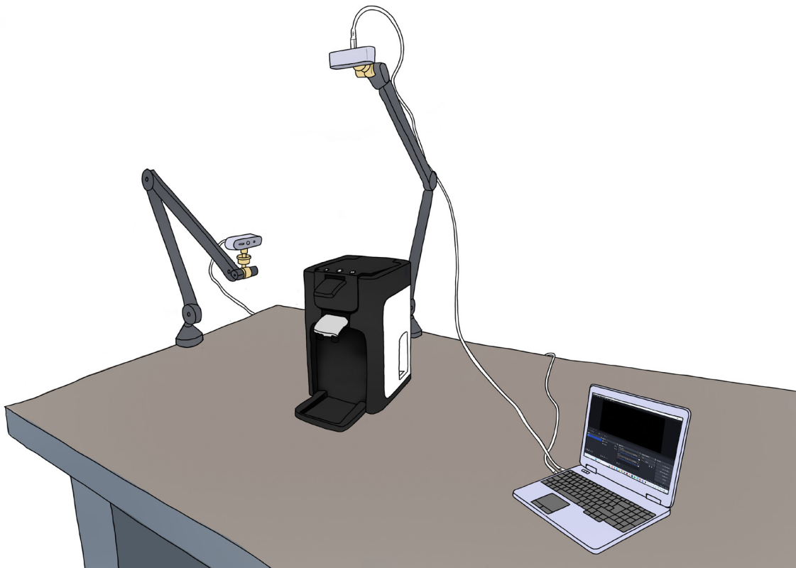
Figure 6: Setup to capture disassembly and reassembly steps
