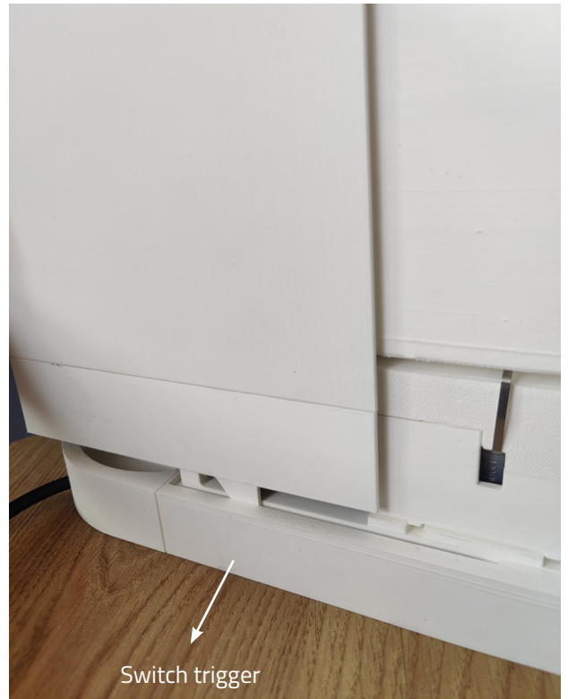
Figure 35: Switch trigger that presses against the PTM switch
