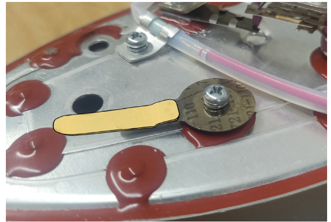
Figure 66: The proposed redesign for the bimetal in the second image to provide sufficient vertical movement
