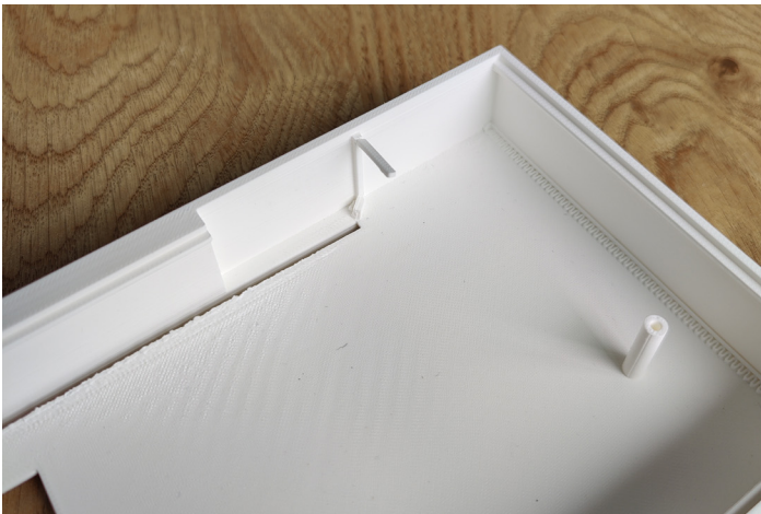
Figure 131: Broken slot for PTM switch and temporary measure used to hold it in place
