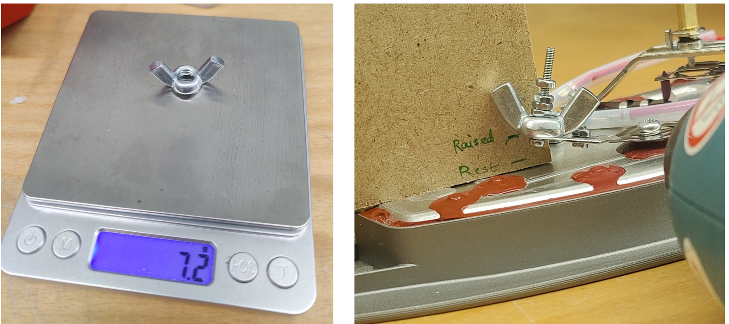
Figure 70: Addition of a 7 gram nut to the bimetal, with no effect on the deflection
