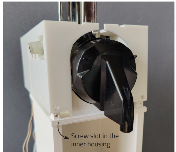
Figure 130: Two threaded connection points were provided to allow the brewing assembly cover to be attached to the inner housing
