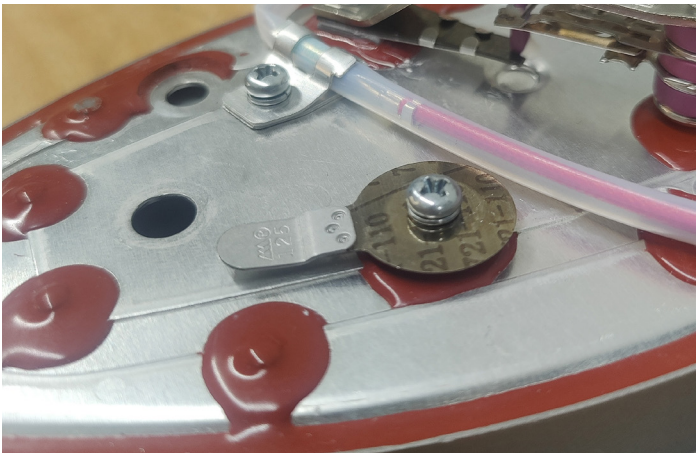
Figure 66: The proposed redesign for the bimetal in the second image to provide sufficient vertical movement
