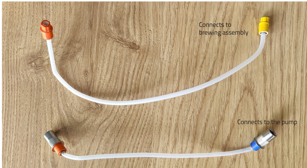
Figure 55: Hoses modified to connect to the components and appropriately colour coded to indicate the orientation of attachment
