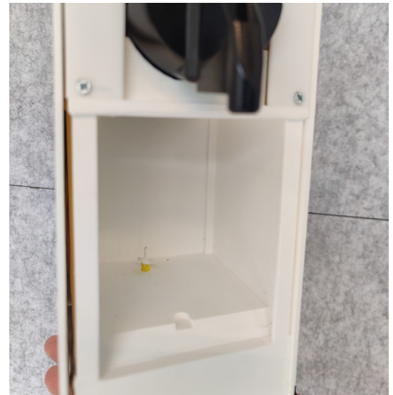
Figure 135: A pin can be inserted to lock the outer housing for the user test
