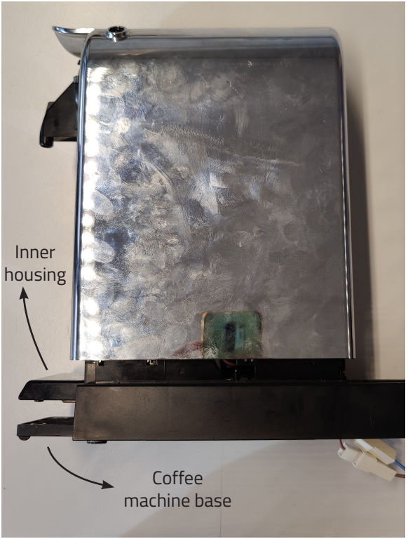
Figure 77: The inner housing is connected to the base in the Magimix. This is clumped in the prototype (Section 5.1)
