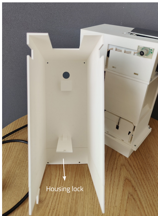
Figure 36: Housing lock used to restrict the outer housing when the boiler is hot
