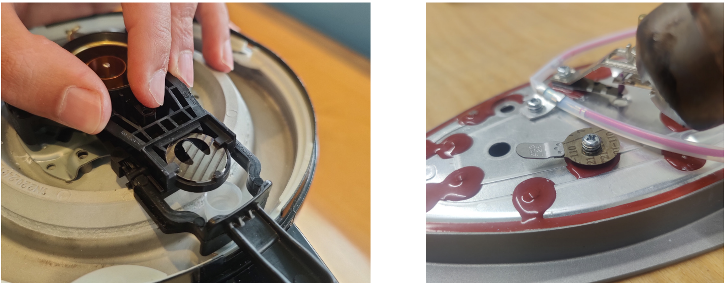
Figure 44: Testing the bimetals used in an electric kettle (left) and steam iron (right) to actuate a mechanism (details in Appendix E)
