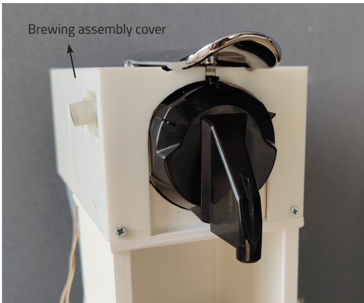
Figure 130: Two threaded connection points were provided to allow the brewing assembly cover to be attached to the inner housing
