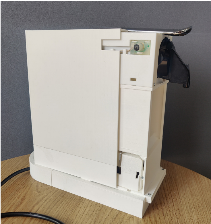
Figure 34: Outer housing slides out once the screws are removed
