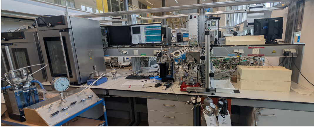
Figure 3.5: Wide-angle view of the experimental lab setup. From left to right: The Booster, Vindum pump station, sensor panel, core holder bench, and data acquisition system are all integrated into a single test rig.
