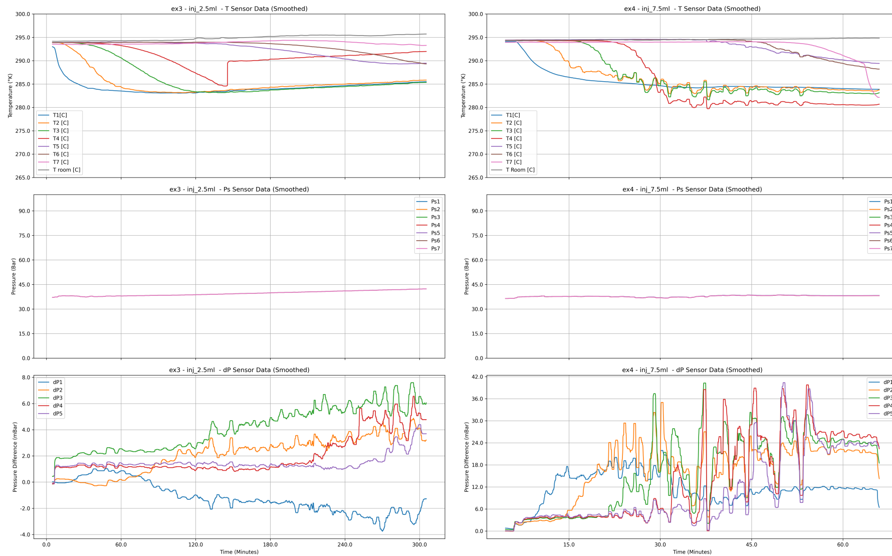
(a) Smoothed sensor data for Experiment ex3: 2.5 mL/min liquid CO 2 injection, Inlet BPC: 30 bar, Outlet BPR: 38.5 bar. (b) Smoothed sensor data for Experiment ex4: 7.5 mL/min liquid CO 2 injection, Inlet BPC: 30 bar, Outlet BPR: 38.5 bar.
