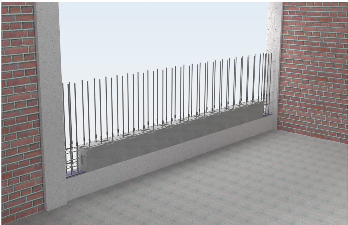
Figure J.12 - Step 12: In this step, the exposed end of the longitudinal rebar is extended using a mechanical rebar coupler, allowing the next rebar segment to be connected. This maintains reinforcement continuity between block layers and enables the next sequence of modular blocks, stirrups, and shear dowels to be installed.
