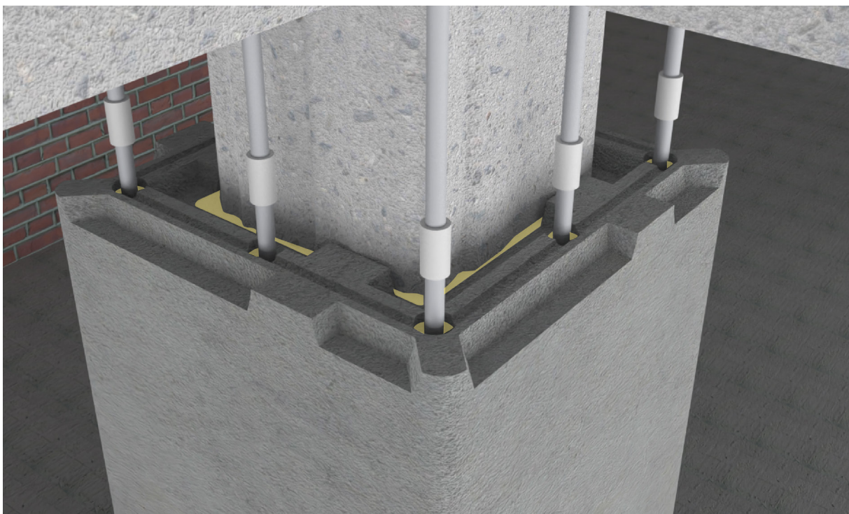
Figure 6.9: Application of the non-shrink grout (highlighted in yellow) ensuring proper shear/load transfer between the old column and the new retrofit elements (author's own work)
