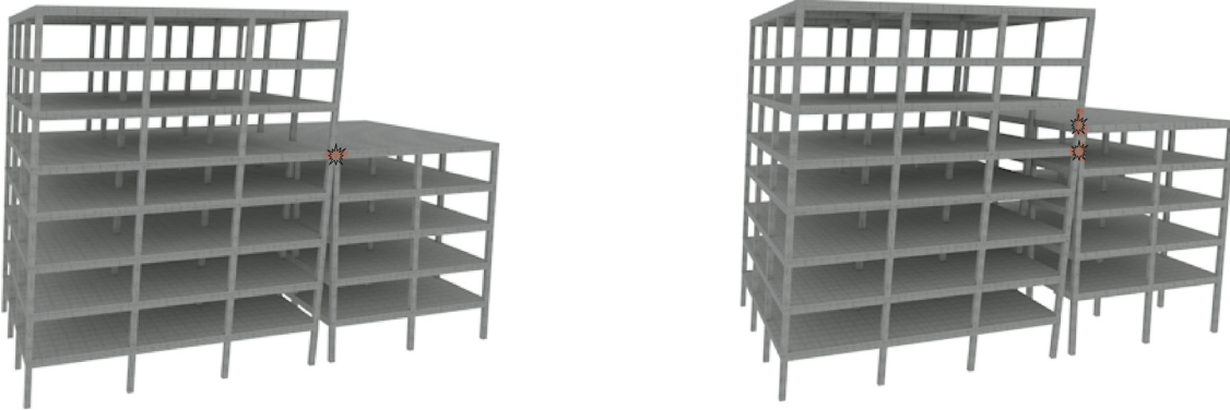
Figure 3.28: The effect of pounding between buildings having similar storey heights (left) and different storey heights (right) (author's own work)
