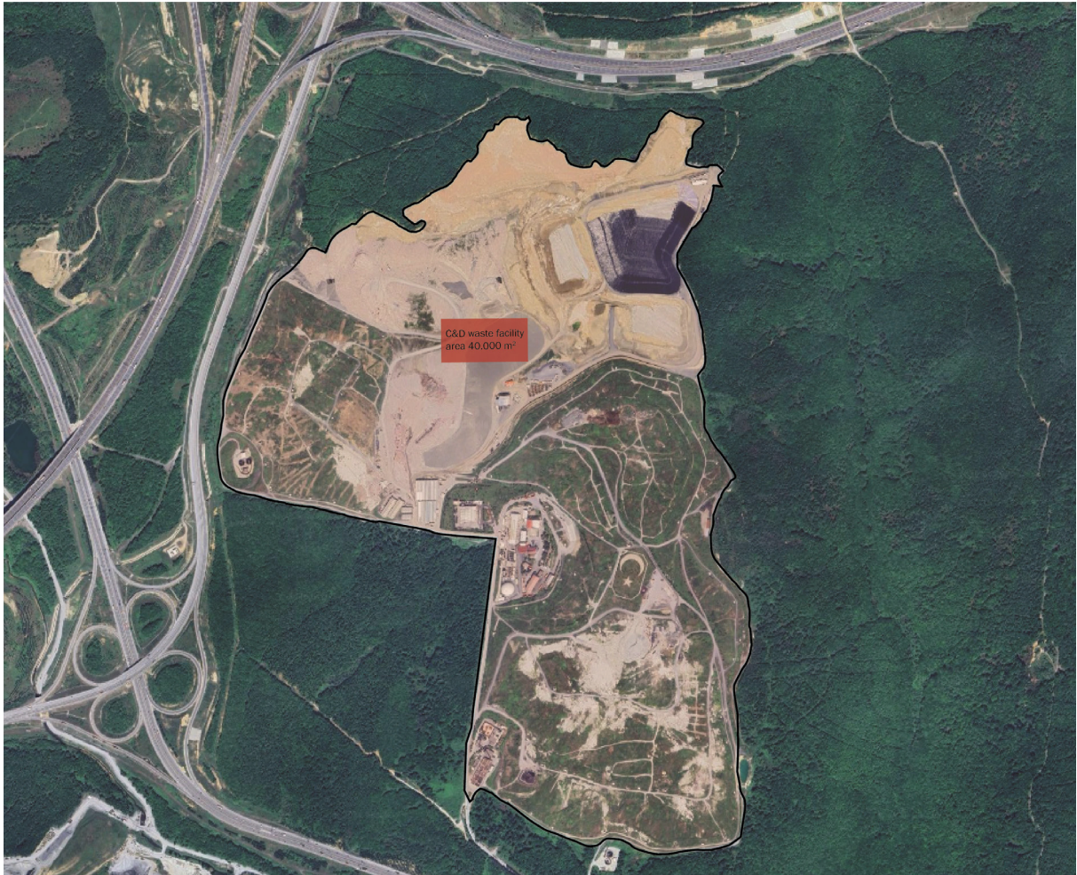
Figure 4.2: The comparison between the current Götürk-Odayeri landfill-incineration facility area (bright-red) and the estimated necessary area for a C&D waste recycling facility plant with a 100 t/h capacity (image adapted from Google Earth, n.d.)
