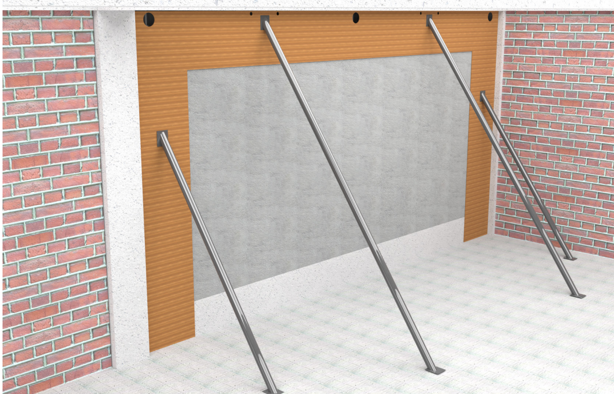
Figure J.18 - Step 18: This pouring is done by applying a timber framework which is stabilised by using adjustable push-pull props. Furthermore, three Ø100 mm holes are applied for the insertion of the cast-in-place concrete, while four smaller Ø30 mm air vents are also made to allow trapped air to escape during pouring, preventing air pockets and incomplete filling of the formwork.
