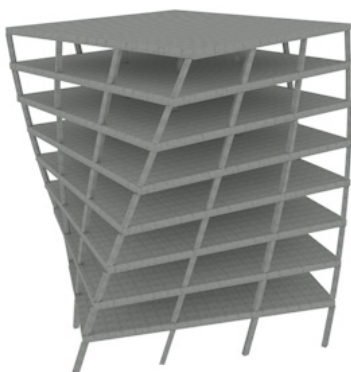
Figure 3.27: The effect of torsional instability on structure (left; author's own work) and as seen through a plan view (right) (Gokdemir et al., 2013)
