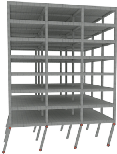
Figure 3.26: The soft-storey effect illustrated with the corresponding plastic hinge formation (left) and seen in the reconnaissance study (right) (Sezgin et al., 2024)
