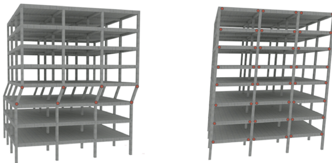
Figure 3.24: The difference between weak-column strong-beam mechanism (right) and strong column weak beam mechanism (left) with the corresponding plastic hinge formation shown in red (author's own work)
