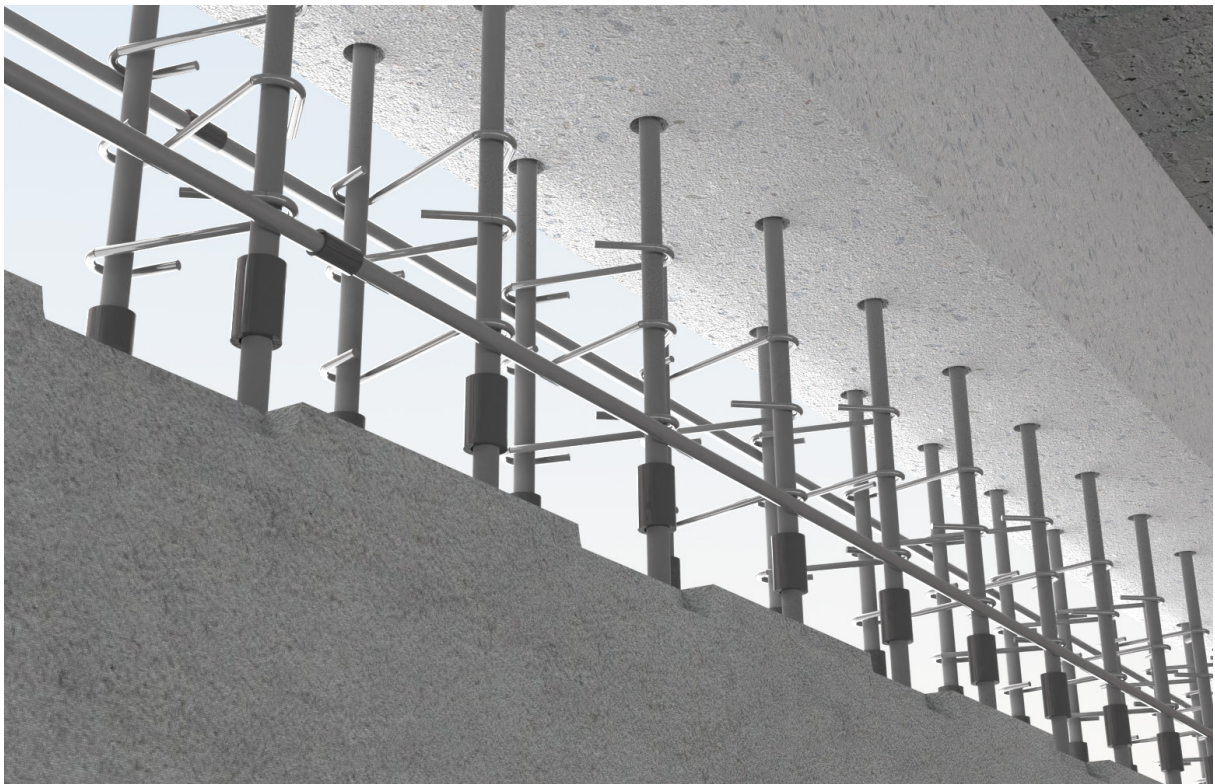
Figure J.16 - Step 16: After the longitudinal rebar is inserted, the couplers can be turned back into its intended place, connecting the longitudinal rebars into one continuous element.
