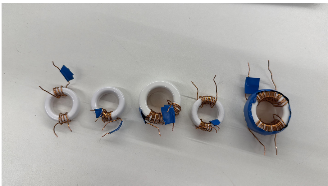
Figure 5.1: Toroids, from left to right: TM 5, TM 5 layered, TL 13 layered, TM 10, TL 20
