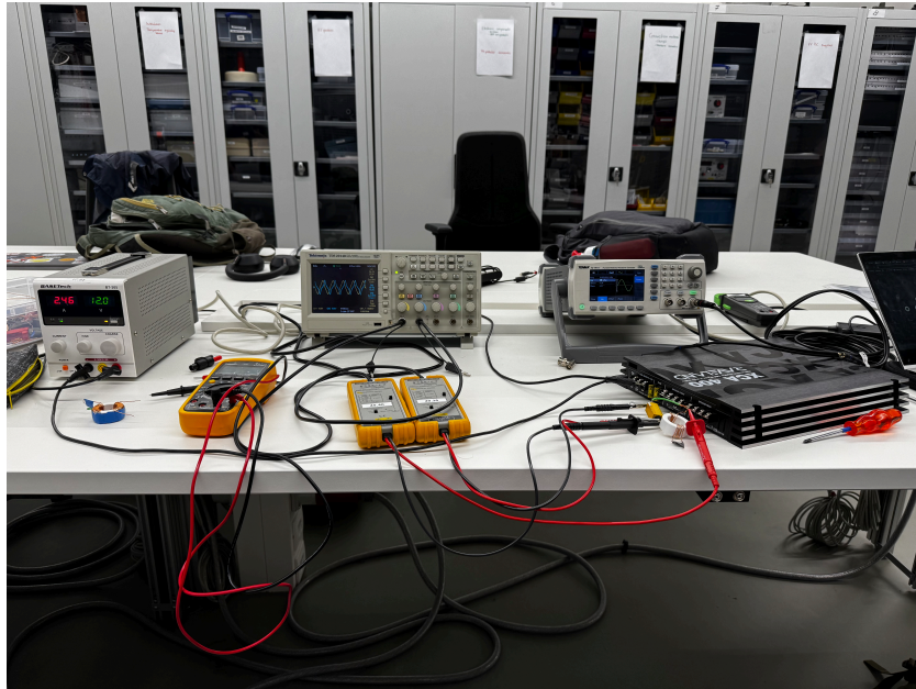
Figure 5.5: Measurement setup for core saturation.
