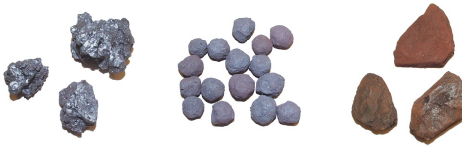
Figure 1.4 The main components of the ferrous mixture: sinter (left), pellets (middle), and lump ore (right) [6].
