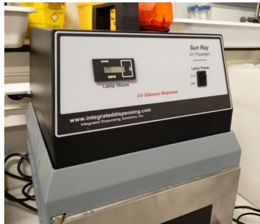
*Image 6 – Close-up of UV Floodlight used for crosslinking in the Biomaterial laboratory at TU Delft.*
