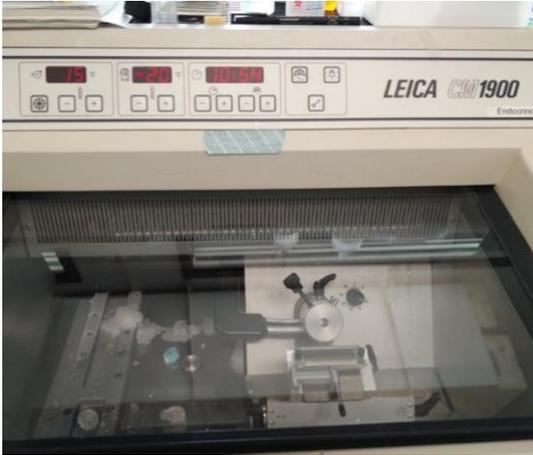
*Image 1 - Leica Cryo-slicer at Leiden University Medical Center. This machine was used to slice 60 $\mu$ m slices for the Atomic Force Microscopy.*
