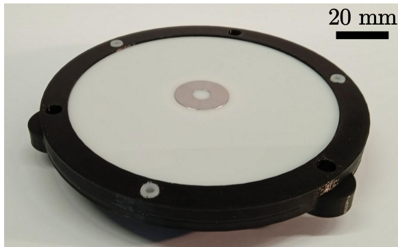
Figure C.7: Photo of the adapted ground plate comprising an aluminium ring with PMMA inserts (white).
