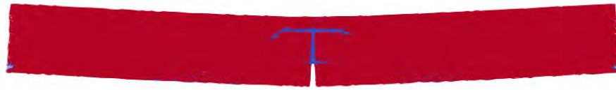
Figure 4.12: Damaged lattice output beam sample 34 showing concrete failure. Deformation scaling factor x30. Red indicating intact elements, blue failed elements.
