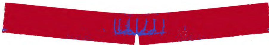
Figure 4.8: Damaged lattice model beam sample 49 showing partial failure. Deformation scaling factor x30. Red indicating intact elements, blue failed elements.
