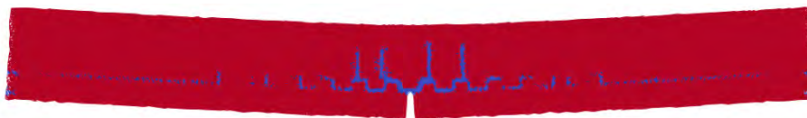
Figure 4.14: Damaged lattice output beam sample 24 showing interface failure. Deformation scaling factor x30. Red indicating intact elements, blue failed elements.
