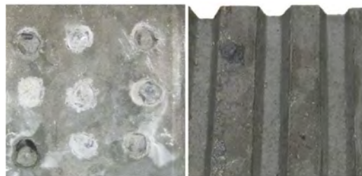
Figure 3.22: Left: holed interface, right: grooved interface, from [38].
