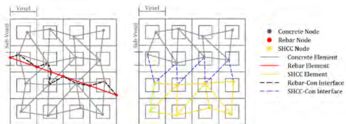
Figure 2.13: Lattice model aspects for reinforced concrete (left) and concrete-SHCC with an interface (right), retrieved from [2].
