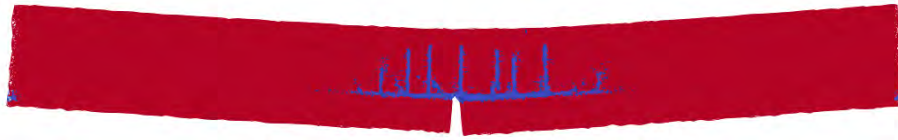
Figure 4.10: Damaged lattice model beam sample 17 showing interface failure. Deformation scaling factor \times 30 . Red indicating intact elements, blue failed elements.
