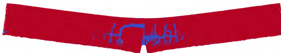
Figure 4.18: Deformed damaged lattice output beam sample 65 showing concrete failure. Deformation scaling factor x30. Red indicating intact elements, blue failed elements.
