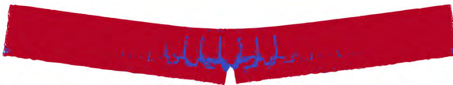
Figure 4.16: Damaged lattice output beam sample 32 showing partial failure. Deformation scaling factor x30. Red indicating intact elements, blue failed elements.
