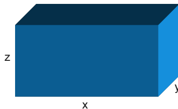
Figure A.1: The homogeneous system is a small cuboid, with mono-energetic neutrons and isotropic scattering. The cuboid is placed in vacuum.
