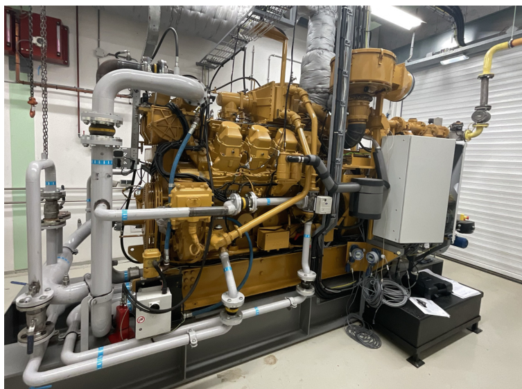
Fig. 2. The HD Marine four-stroke SI engine experimental setup in Den Helder, Netherlands (Image courtesy MENENS project.)
