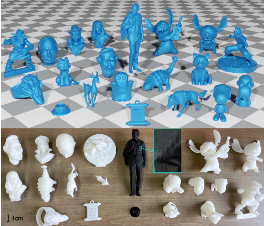
Figure 5.7: Test set consisting of models from Shen et al. (2022) , which were 3D printed and subsequently scanned to capture real-world noise characteristics. The zoom-in highlights printing artifacts, such as the vertical lines visible on the Suit Man model.
