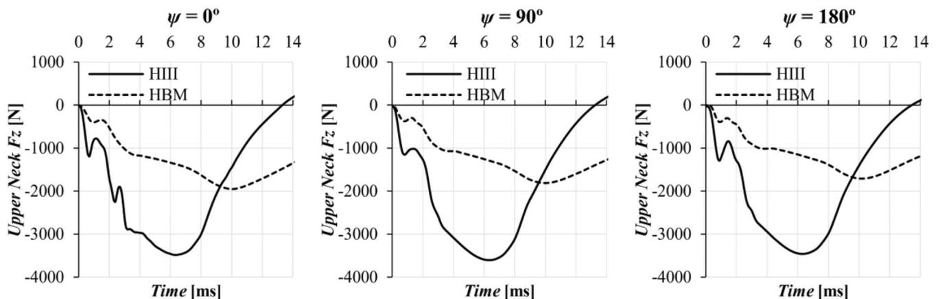
Comparison of upper neck force in Z-direction between the Hybrid III and the human body models at various impact conditions and at 196 J impact energy (equivalent to 18 m/s impact velocity)
