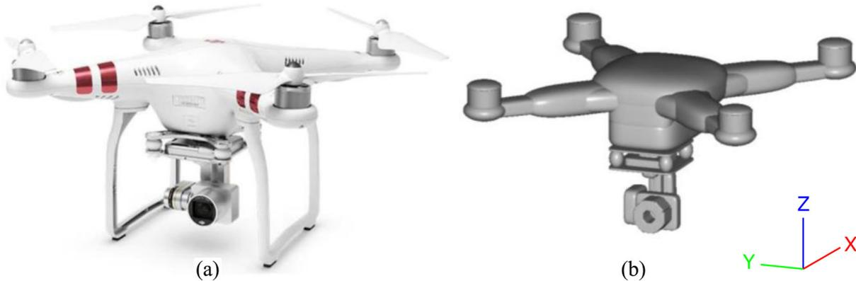
**Figure 1.** DJI Phantom III UAS used in impact modelling: (a) real-world system and (b) multibody system (MBS) model developed in MADYMO<sup>11</sup>. The two landing skids are neglected in the MBS model since they are such flexible that their impact effect is negligible [11].
