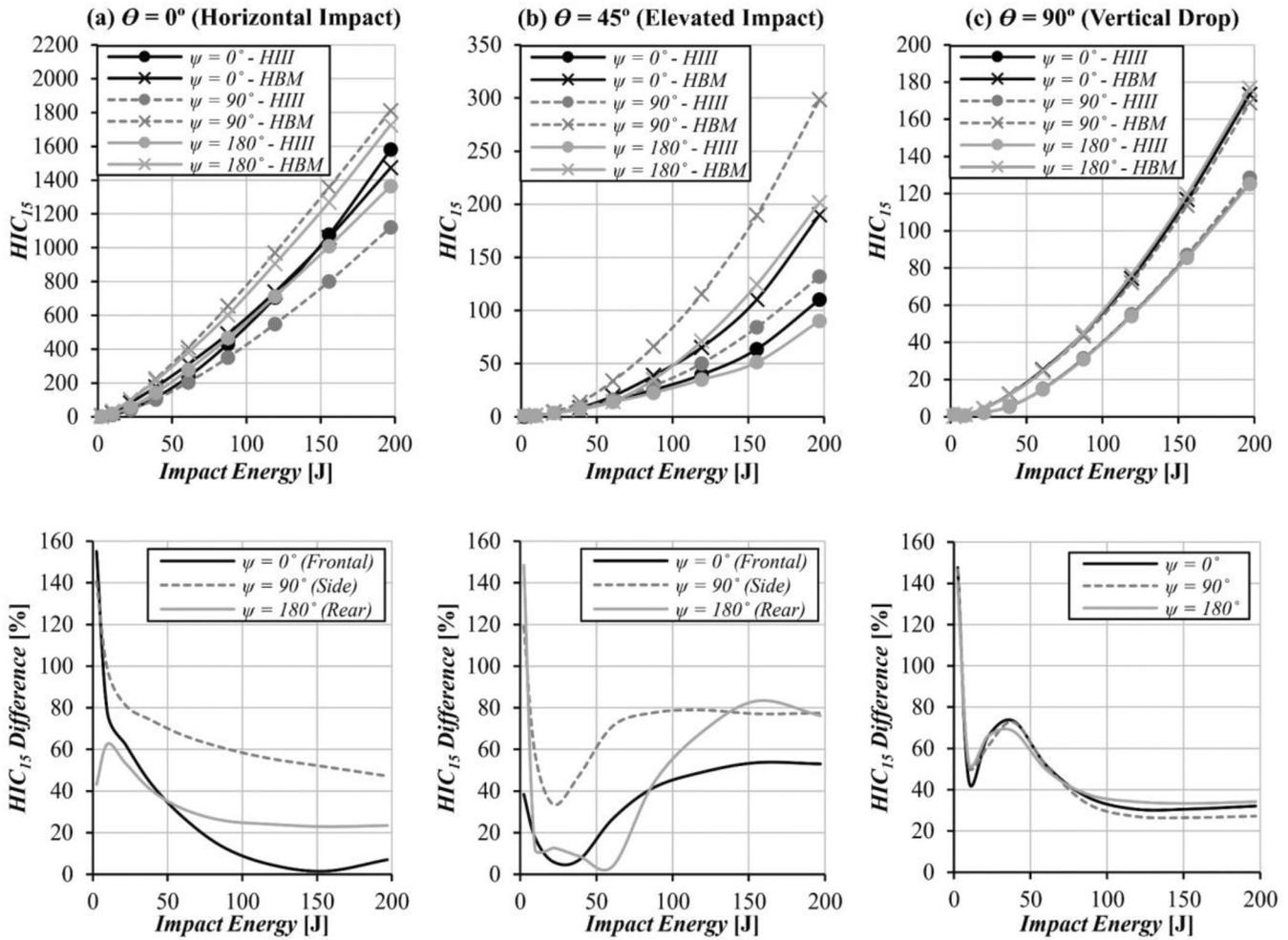
**Figure 6.** Comparison of  $HIC_{15}$  between the Hybrid III and the human body models (upper figures) and the percentage in  $HIC_{15}$  of Hybrid III dummy relative to the 100% for the human body (lower figures) at different impact energy,  $\theta$ , and  $\psi$ .
