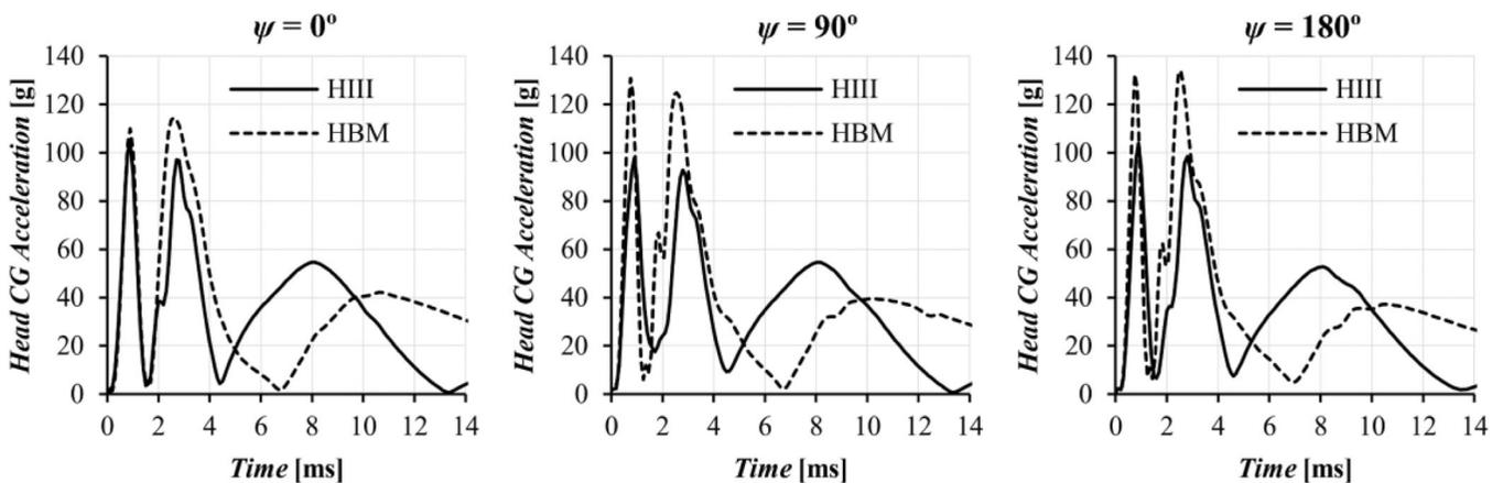
Comparison of head CG acceleration between the Hybrid III and the human body models at various impact conditions and at 196 J impact energy (equivalent to 18 m/s impact velocity)
