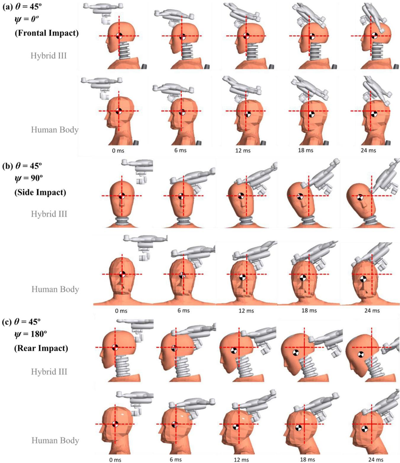
**Figure 4.** Comparison of impact sequences between the Hybrid III and the human body for  $\theta = 45^\circ$  (elevated impact) and  $\psi = 0^\circ, 90^\circ$  and  $180^\circ$  at 196 J impact energy (equivalent to 18 m/s impact velocity).
