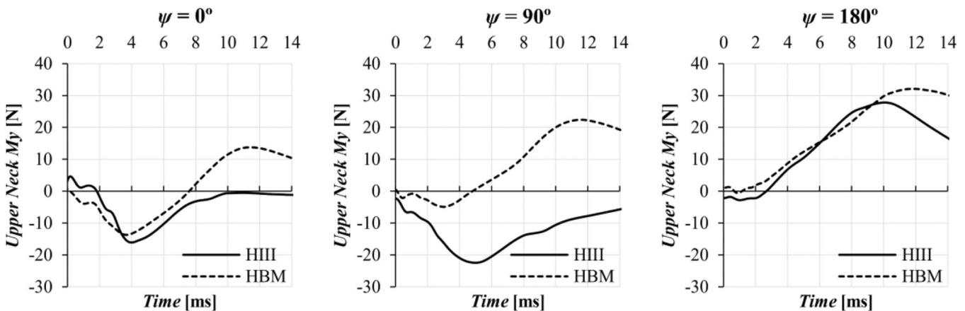
Comparison of upper neck moment about Y-axis between the Hybrid III and the human body models at various impact conditions and at 196 J impact energy (equivalent to 18 m/s impact velocity)
