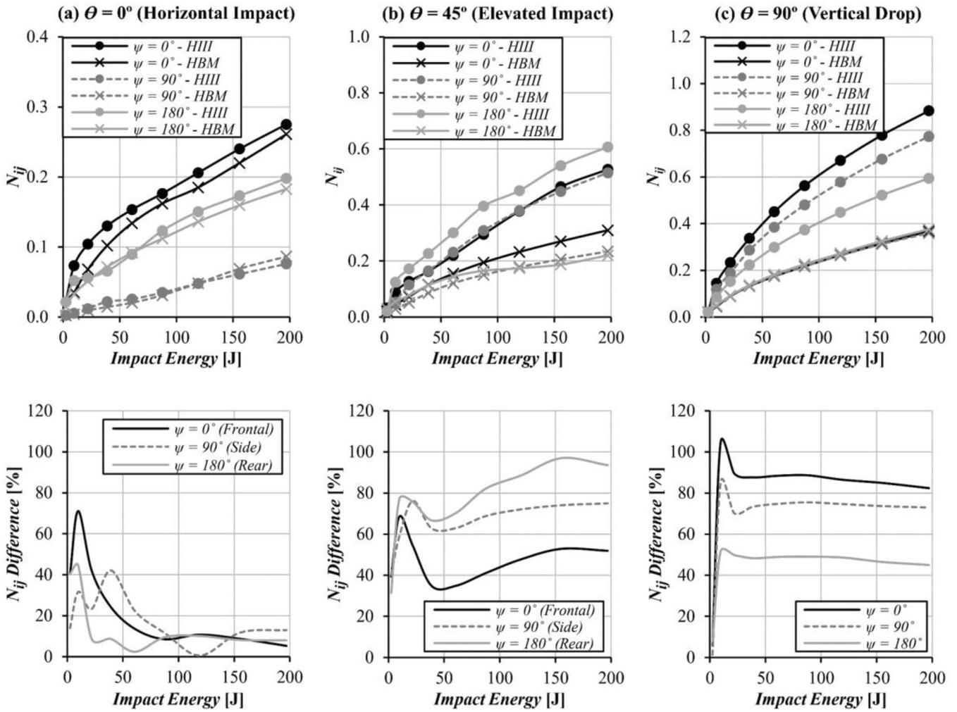
**Figure 7.** Comparison of  $N_{ij}$  between the Hybrid III and the human body models (upper figures) and the percentage in  $N_{ij}$  of Hybrid III dummy relative to the 100% for the human body (lower figures) at different impact energy,  $\theta$ , and  $\psi$ .
