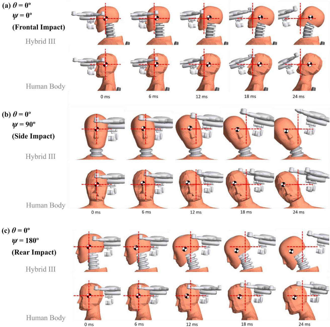
**Figure 3.** Comparison of impact sequences between the Hybrid III and the human body for  $\theta = 0^\circ$  (horizontal impact) at  $\psi = 0^\circ, 90^\circ$  and  $180^\circ$  at 196 J impact energy (equivalent to 18 m/s impact velocity).
