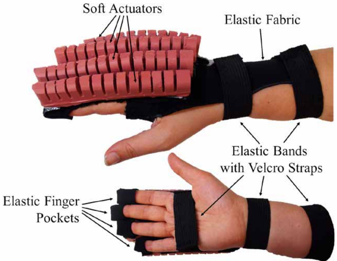
Figure 13: Pneumatic Bending Actuators by Polygerinos 2013
