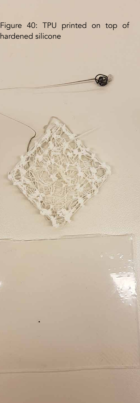
Figure 41: TPU printed on top of hardening silicone
