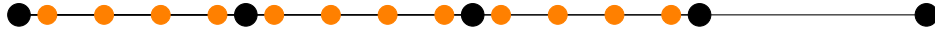
Figure 3.2: Discretized domain \Omega \in \mathbb{R} and initial configuration \Omega_0 \in \mathbb{R} consisting of five degrees of freedom and equally distributed particles.
