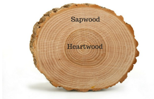
Figure 2.2: Cross section of a tree with a clear distinction between the darker heartwood and the lighter sapwood [21]
