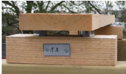
Figure 4.12: Reference element for climate exposure – horizontally exposed spruce board without moisture traps [17]
