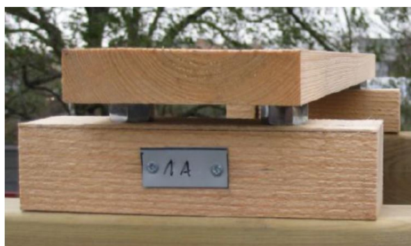
Figure 5.2: Swedish reference situation, spruce board above ground contact.
