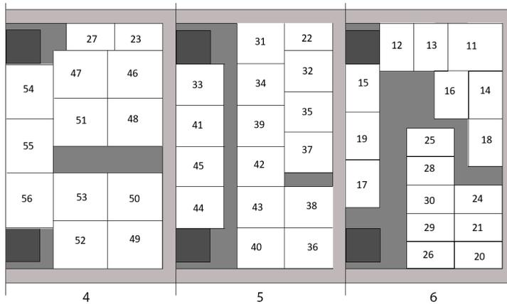
Figure 3.30: A manually created layout plan of deck 4, based on the layout generated by WARGEAR. All spaces meet their required area in the improved layout.
