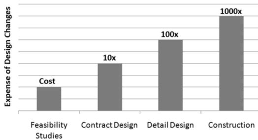
Figure 1.5: Estimates of change costs during different stages of design for naval vessels (Kana et al., 2016; Keane & Tibbitts, 1996)
