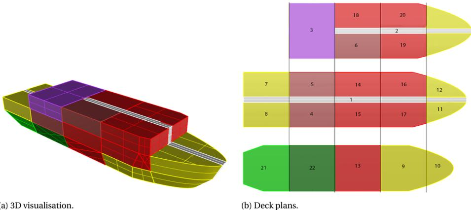
Figure 3.1: Arrangement of the notional surface vessel used in Case Study 1. See Appendix B.2 for details.
