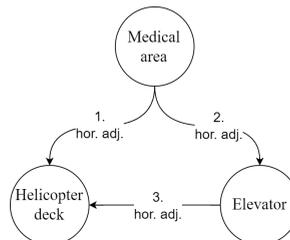
Figure 5.1: Required connectivity between a medical room and a helicopter deck, comprising a compromise between interaction 1 and interactions 2 and 3.
