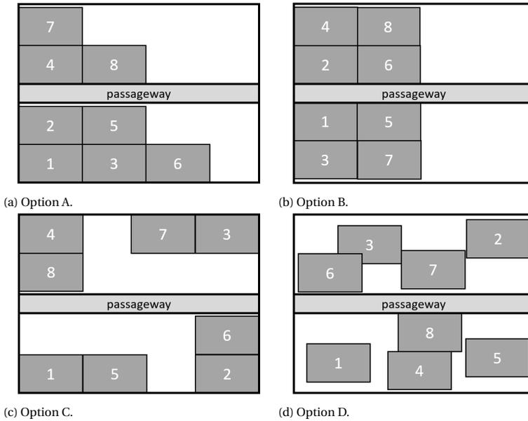
Figure 2.13: Visualisation of space position selection options in an example of a compartment with a central passageway
