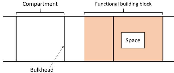
Figure 2.3: Visual explanation of the subdivision of a deck, presented in a top-down view. An FBB overlapping multiple compartments is shown (Le Poole et al., 2019).
