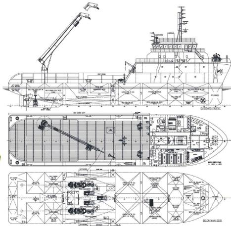
(d) High level of detail 2D GAP (Seaboats.net, n.d.)
