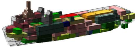
(b) Low level of detail 3D arrangement (Van Oers, 2011a)
