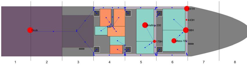
Figure 3.31: Arrangement of deck 3 in the selected layout with overlaying network representation, as well as an indication of locations where functional or logistical waiting time is created (red circles), based on the output of the queueing method.
