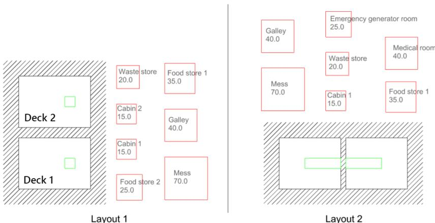
Figure 4.7: Visualisation of the two layouts (black) and corresponding staircase or passageway (green) and systems (red). The numerical value in each system is its required area [ $m^2$ ]. The current area of systems shown equals the required area. Compartments are sized 14m by 10m (Layout 1) and 12m by 10m (Layout 2).
