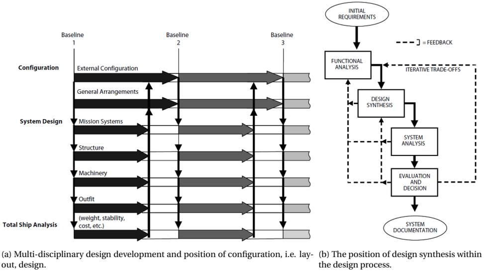
Figure 1.10: Ship design process and role of layout generation (Lamb, 2003).
