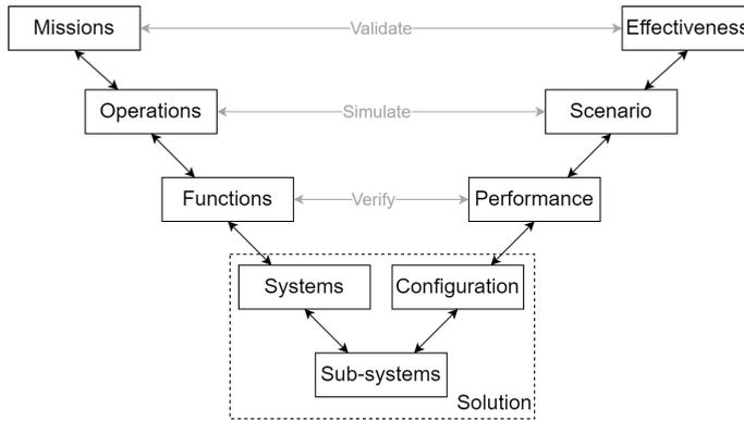
Figure 1.2: Systems engineering V diagram, adapted from (Duchateau, 2016).
