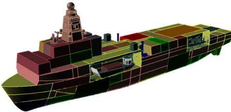
(c) Medium level of detail 3D arrangement (Van Oers, 2011a)
