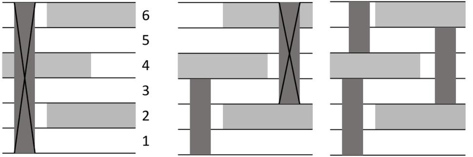
(a) The required staircase cannot be placed and needs to be split, as indicated by the black cross.
