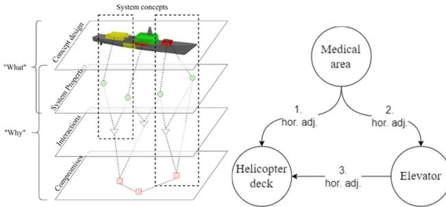
**System Concept:** contains a (sub)set of the layout (or it's systems) and the design rationale behind this (sub)set + rationale behind the concept and can be related to other design rationale, e.g. a compromise between two propulsion concepts.
