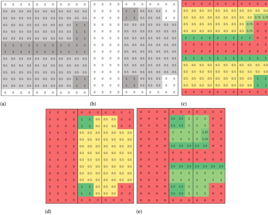
Figure 2.8: Creating a staircase positioning matrix for a two-deck, three-compartment test case. (a) Deck 1 with an L-shape passageway and a small lobby. (b) Deck 2 with an irregular shape and two lobbies. (c)  $SPM_1$  for deck 1. (d)  $SPM_2$  for deck 2. (e) Aggregated FSPM for the two decks, where higher values represent more preferred positions for staircases.
