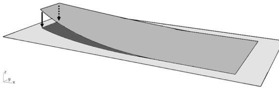
Figure 3.8: Projecting a curved deck to a flat deck plane.
