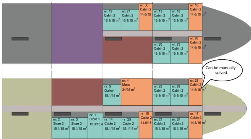
Figure 3.4: Upper two decks of the best performing layout from Case Study 1b (ID 58). The lowest deck was properly arranged
