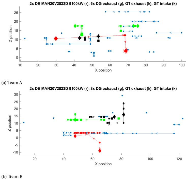
Figure 5.19: Example of changes to positions of systems due to the addition of other systems: The effect of the change of the propulsion concept on the layout of exhausts (Design Session 1 versus 2). Color codes: r = red, g = green, k = black.
