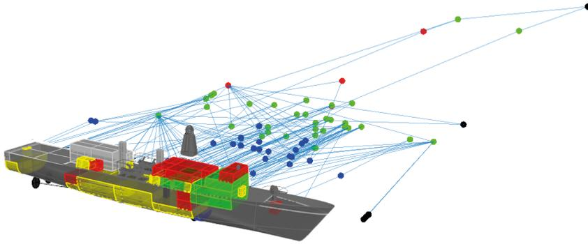
(a) Rationale network overlaying the OPV concept design. System nodes outside the concept design represent systems that have not yet been arranged.
