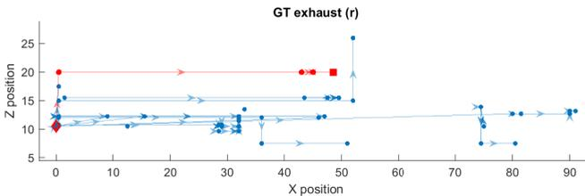
Figure 5.18: Example of a network of system positions (nodes) over time. Arrows indicate how systems are relocated. One system is highlighted (red) with its start (diamond) and end (square) positions indicated.
