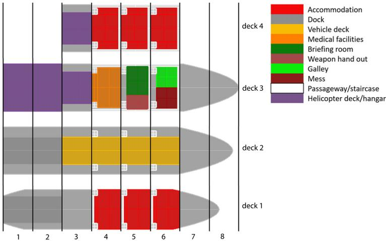
Figure 3.27: A functional arrangement of the notional LPD.
