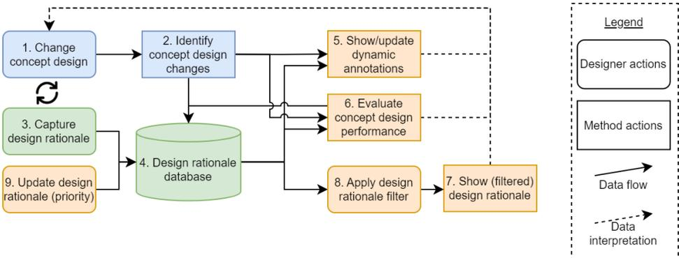
Figure 4.4: Schematic overview of the developed method for ship layout design. Blue: support and identification of manual design changes. Green: design rationale capturing and storage. Orange: design rationale retrieval and feedback.
