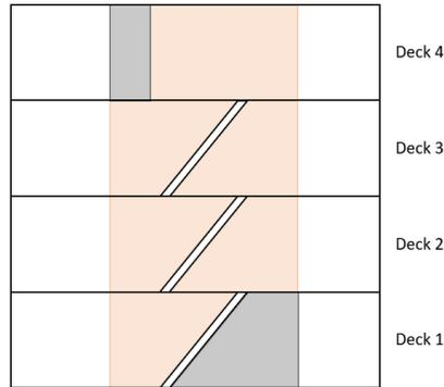
Figure 3.10: Difference between open area required around ship staircases in reality (orange) and area arranged by WARGEAR (orange and grey).
