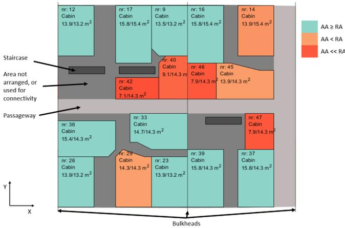
(a) The detailed layout as generated by WARGEAR, scoring  $F = 27.1$
