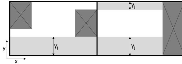
Figure 2.6: Top view of a two-compartment example on main passageway selection. Legend: *dark grey, black cross*: blocked area; *light grey*: available area for the main longitudinal passageway. The *two-headed arrow* indicates feasible  $y_j$ .
