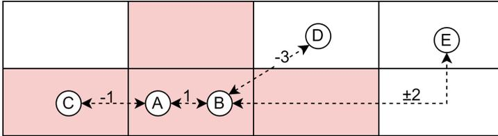
Figure 3.13: Visual representation of implemented interaction types. A–B: Compartment adjacency; A–C: Compartment separation; B–D: minimum radial separation; B–E: minimum/maximum Manhattan distance.
