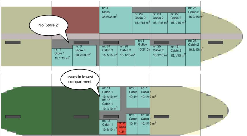
(b) Lowest two decks of the best-performing layout that misses one space from Case Study 1a (ID 55). The upper deck is arranged similarly as layout ID158, Figure 3.3a.
