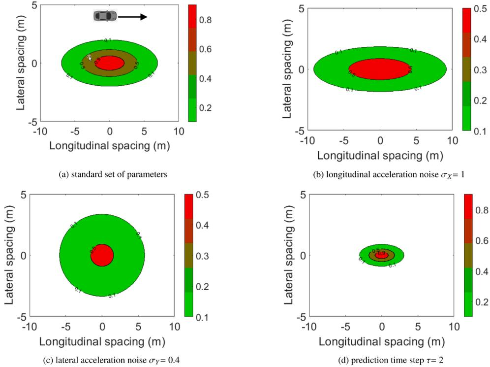
Fig. 2. Collision likelihood contours around  $n$ , for a subject travelling at the same speed in forward direction: (a) with standard set of parameter values,  $n$  with longitudinal acceleration noise  $\sigma_\chi = 0.7$  and lateral acceleration noise  $\sigma_\gamma = 0.2$  prediction time step  $\tau = 3$ ; and (b), (c) and (d) with a change in value of the parameter specified in the subcaption.
