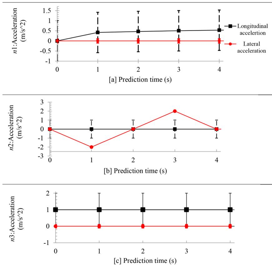
Fig. 11. The trajectory plans of the neighboring vehicles *n1* (a); *n2* (b) and *n3* (c) represented in terms of the expected acceleration ( $\hat{A}_X(t_k)$ ) as square black markers and  $\hat{A}_Y(t_k)$  red dots and the error limits defined by the acceleration noise. (For interpretation of the references to color in this figure legend, the reader is referred to the web version of this article.)
