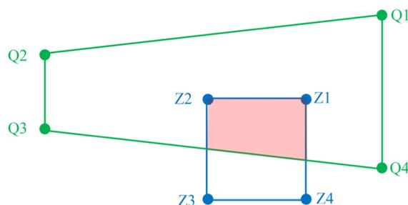
**Fig. 14.** Geometric representation of the polygons Q, Z and their overlap O (area shaded in pink), used for the crash probability estimation in Algorithm A.1. (For interpretation of the references to color in this figure legend, the reader is referred to the web version of this article.)
