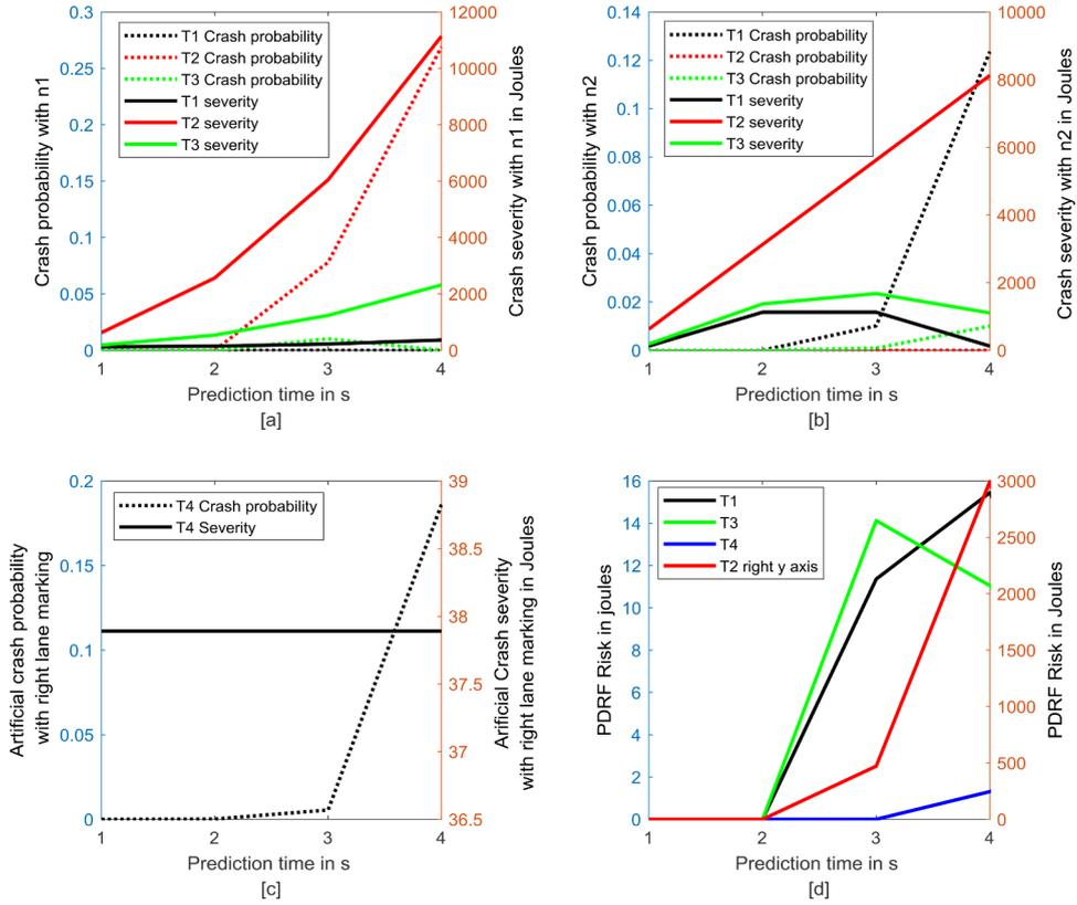
**Fig. 12.** The multi-step PDRF risk estimates for trajectory plans at a typical lane drop section. The probability and severity of a crash between  $s$  and  $n1$  (a);  $s$  and  $n2$  (b);  $s$  and the right lane marking (c); and the combined PDRF risk along the trajectory plans (d).
