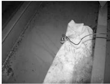
Figure 8.8: Acceleration sensor fitted to the inside of a hull plate
