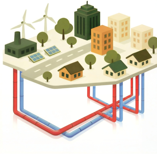
Figure 1.1: District heating network consisting of supply (red) and return (blue) pipelines transporting heated water from producer to consumer and back.
