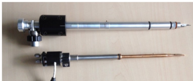
Figure 4.3. A comparison of the shapes of a JEOL and an FEI flowing gas holder.
