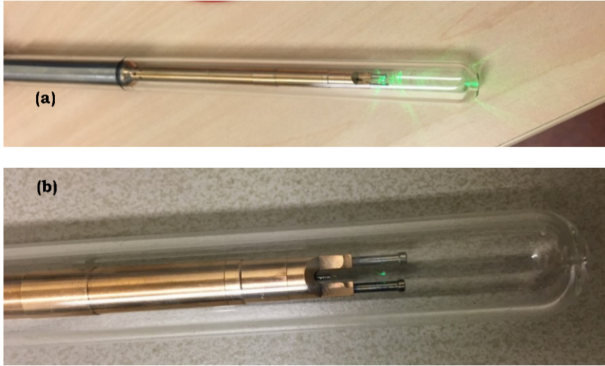
Figure 6.5 TEM holder with Fibre 1 tip after splicing: (a) when the carbon thickness is ~ 5-10 nm. It was not possible to run experiments due to charging and deformation of the tip. (b) The carbon thickness is ~ 50 nm that enables to run experiments.
