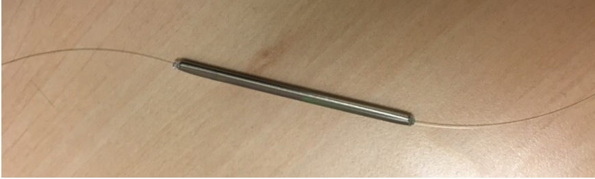
Figure 6.4. Spliced and protected fibres by heat shrink tubing.
