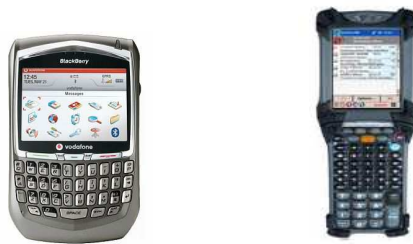
Figure 3.5 Examples of general mobile devices and task-specific mobile devices: Blackberry PDA (left) and Symbol handheld (right)
