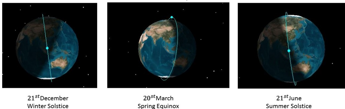
Figure C.1: Representation of a twilight orbit during three different period of the year. The twilight orbit does not enter the Umbra region during the spring equinox and the summer solstice.
