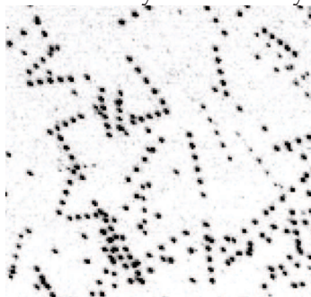
Figure 5: Unprocessed camera image (only background of 340 pixels subtracted, low seeding density, color
