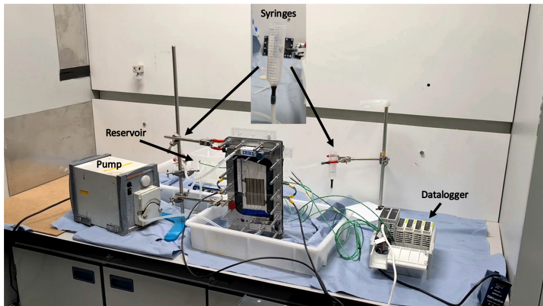
Figure 3.9: The experimental setup inside the fume hood. The electrolyte reservoir can be seen in the background. The syringes affixed on the stands serve as the gas liquid separator. The electrolyzer is shown on the foreground.
