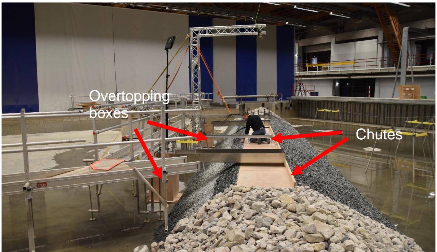
Figure 7. Equipment used to measure the average overtopping discharge.
