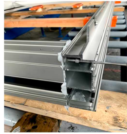
Figure 61: Inserting screws in aluminum profiles (image by Scheldebouw).
