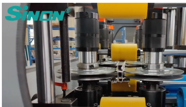
Figure 40: Rolling thermal break process, front view (Sinon, n.d.).
