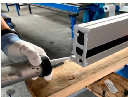
Figure 92: Applying sealant on top of transom profiles (image by author).
