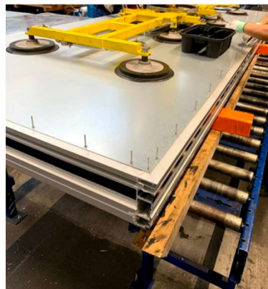
Figure 66: placing all rivets on steel sheet (image by Scheldebouw).
