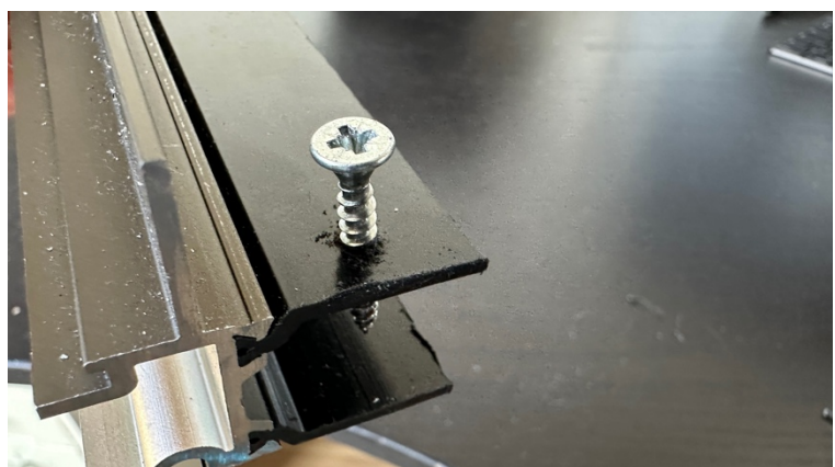
Figure 133: screw drilled through GFRP (image by author).
