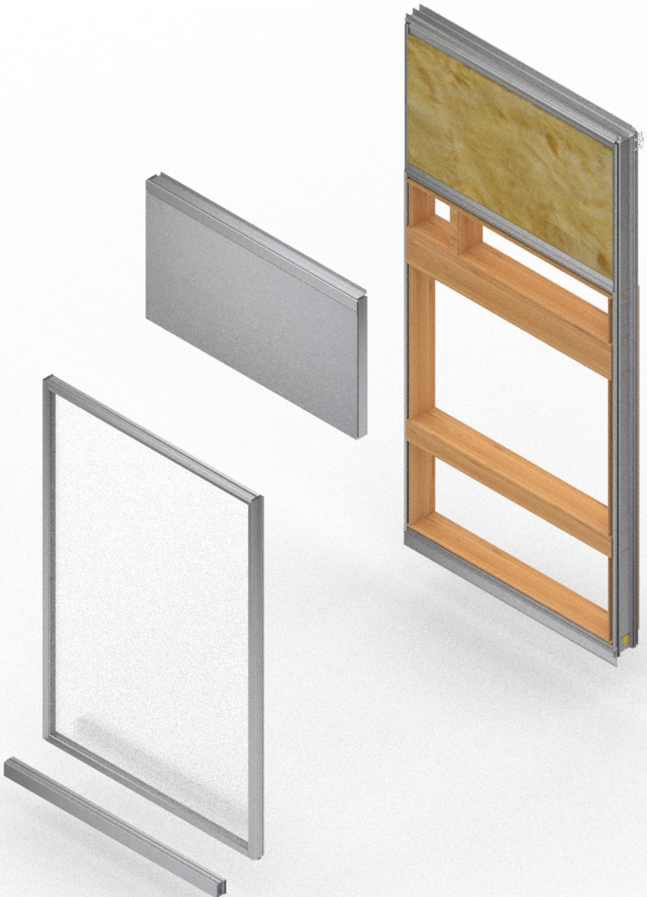
Figure 108: Exploded view carrier frame design ABN AMRO panel (image by author).
