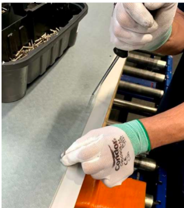
Figure 64: Making small hole for location of rivet (image by Scheldebouw).
