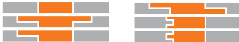
Figure 27: Schematic view of geometries interlocking, leading to obstruction of removal (van Vliet et al., 2021).
