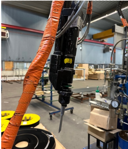
Figure 83: Machine for applying sealant for structural glazing (image by Scheldebouw).
