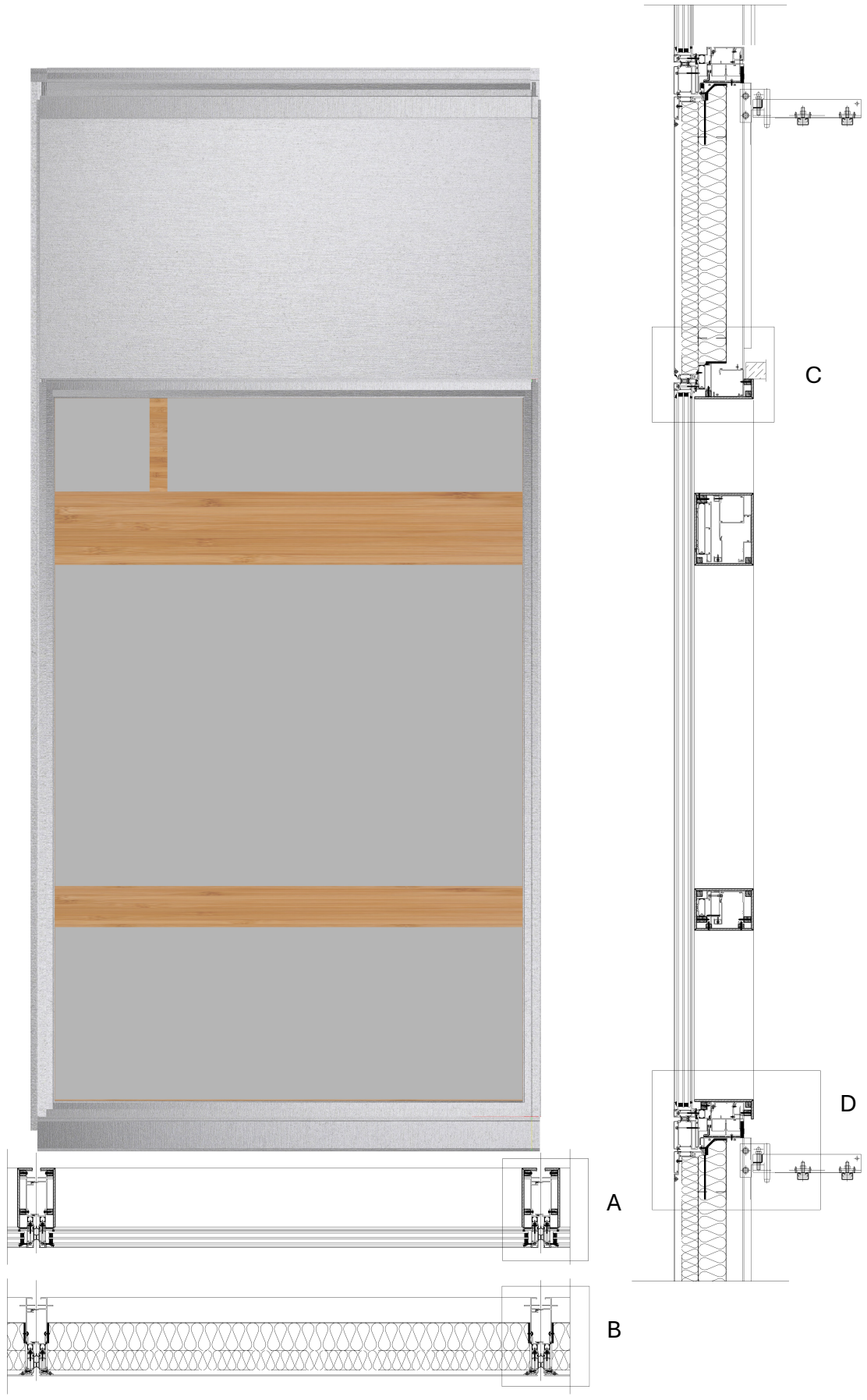
Figure 97: Section 1:20 new design ABN AMRO panel (image by author).
