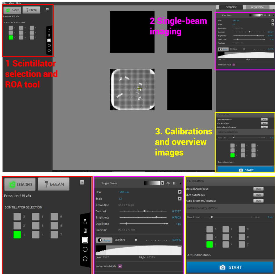
Figure A1: ODEMIS FAST-EM graphical user interface, overview tab. 1: Scintillator selection and ROA definition tools. 2: Single-beam tool. 3: Optical calibration, detector (single-beam) settings, overview image settings.
