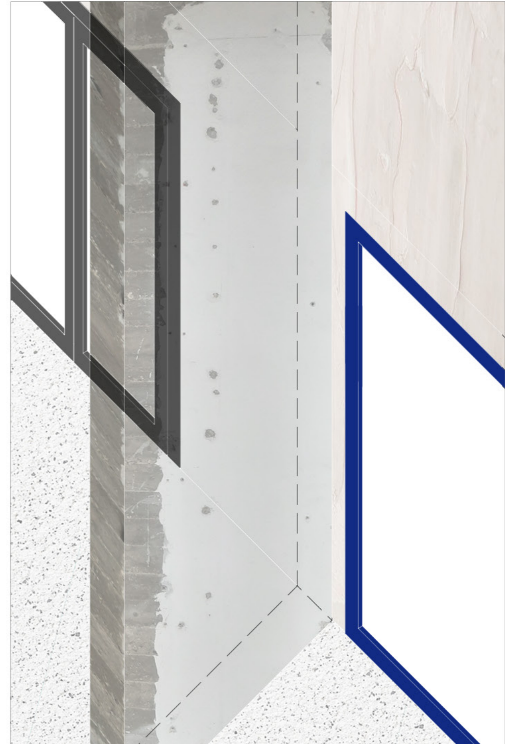
The previous shop's entrances and windows are integrated as internal glazed walls for the art workshops.
