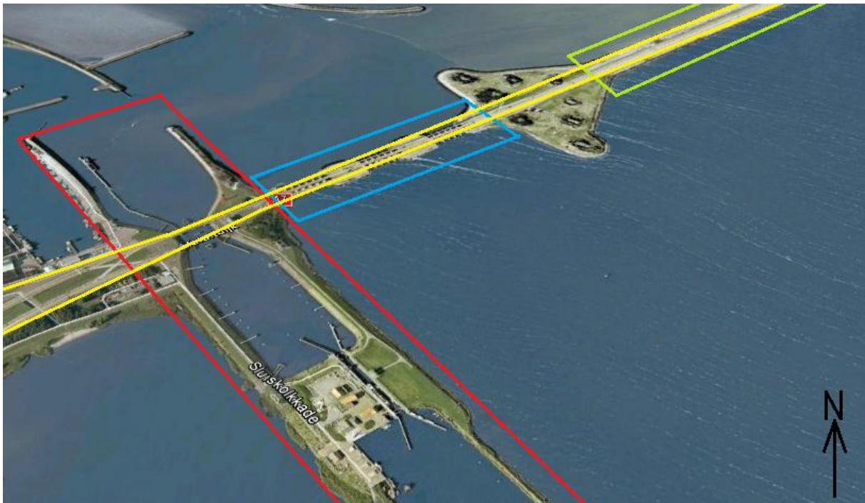
Figure 8-4: A bird view of the current situation of Den Oever which can be divided in a lock complex Stevinsluis (red), discharge sluices (blue), dike (green) and the road connection (yellow) (Source: Google Maps).
