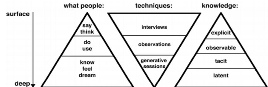
Figure 2.19, the diagram that shows different levels of knowledge about experience are accessed by different techniques from Visser et al.(2005)
