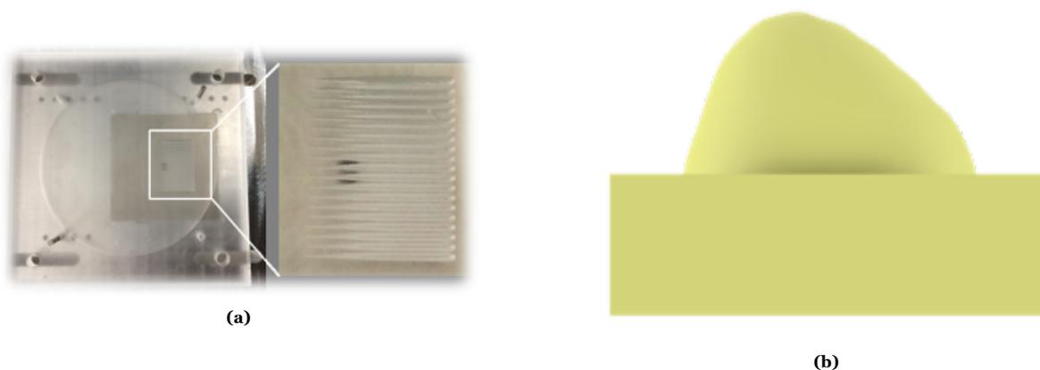
**Figure 1.1:** Examples of solutions addressing the low scanning performance of low density dielectric lenses, with (a) being the dielectric grating wedge in the lens [2] and (b) is an example of a shaped dielectric lens [3].
