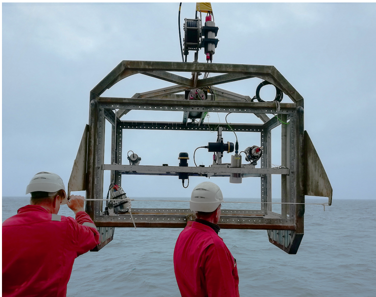
Figure 4.4: Front view of the NIOZ hopper camera.
