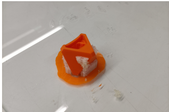
Figure E.1: 3D printed CoastaLock armour unit, right after printing with orange PLA and seethrough PVA.
