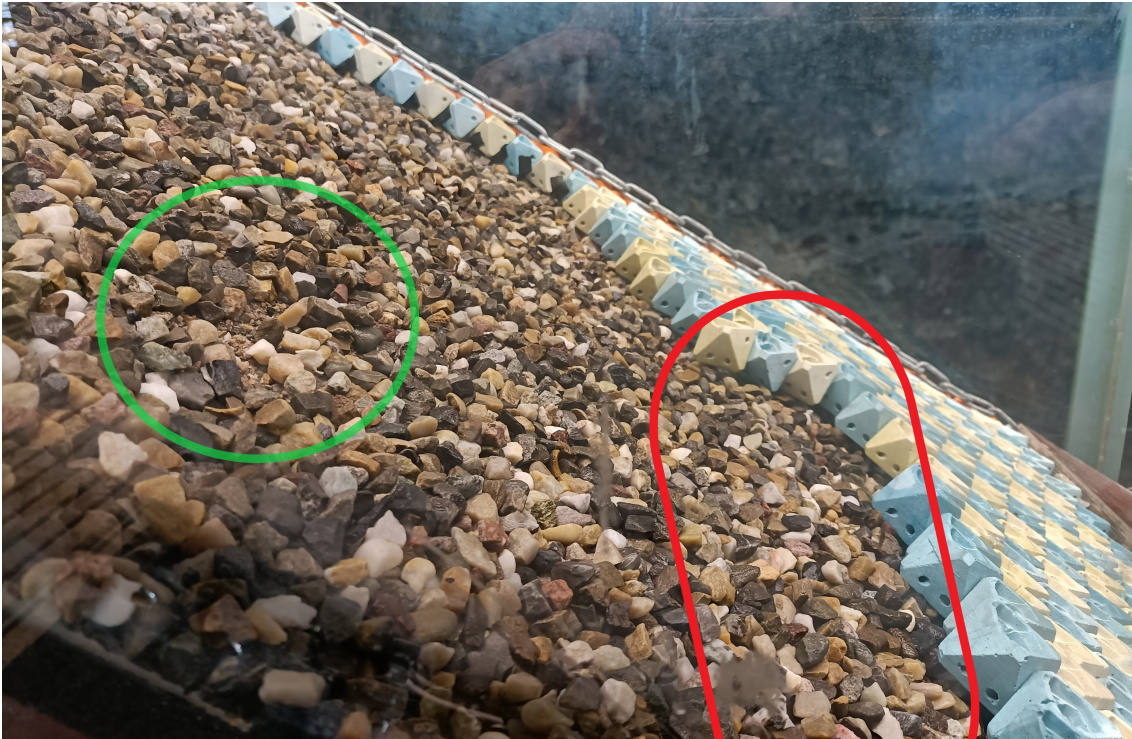
Figure 6.2: Displacement of under layer material due to breathing of the armour layer. Exposure of the core material highlighted in green, accumulation and formation of concave S-profile highlighted in red.
