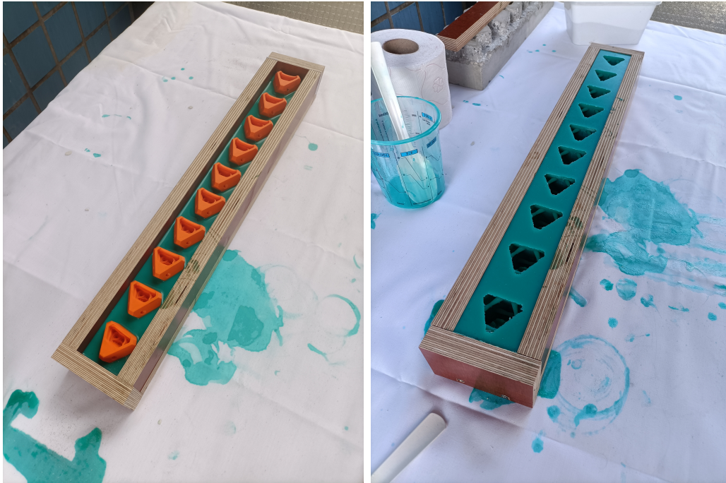
(a) After curing of the first half of silicone. (b) After completion and removal of the units. Please note that the silicone mould has been turned upside down and that the blocks have been extracted from the bottom.
