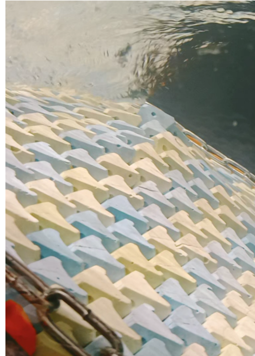
Figure 6.1: Breathing of the CoastaLock armour layer, with layer in raised position.
