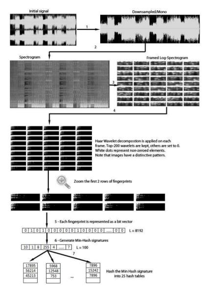
Fig. 2. Sound Fingerprinting Framework (source [17])
