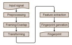
Fig. 1. Steps in Audio Fingerprinting algorithms
