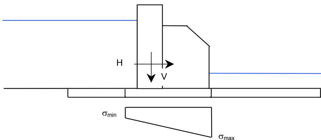
Figure 20: Minimum and maximum pressure under foundation slab
