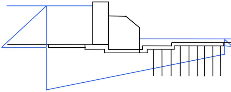
Figure 26: Anchoring the downstream apron
