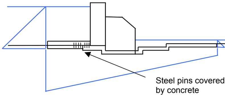
Figure 33: Connection between power house and upstream apron
