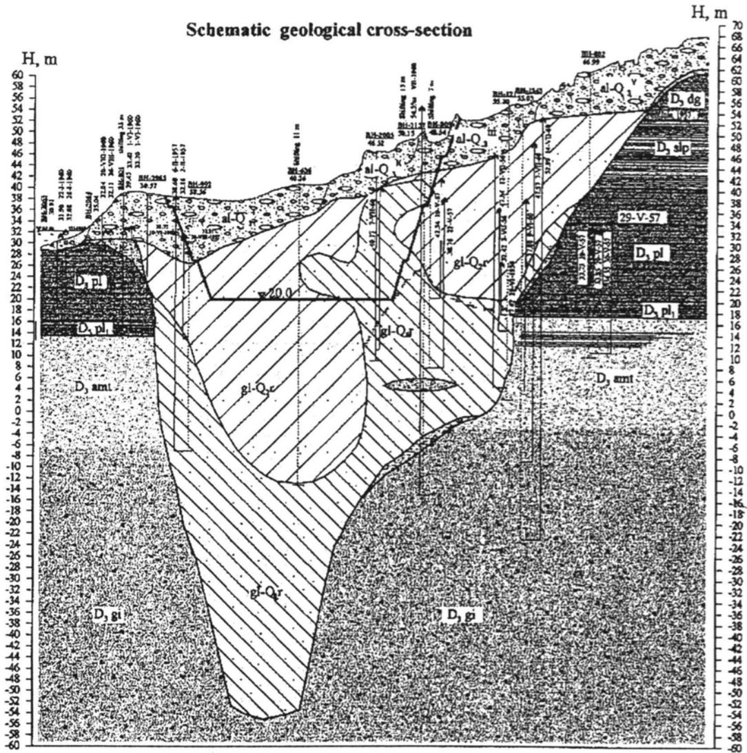
Figure 13: Geological section (longitudinal) across the valley along the axis of the powerhouse<sup>15</sup>
