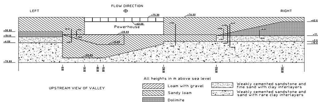
Figure 14: Schematisation of foundation soil at Plavinas in the direction of the dam axis
