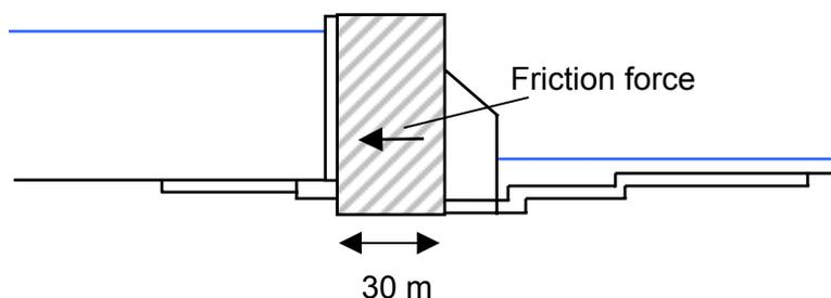
Figure 18: Cross section with support from embankment dams
