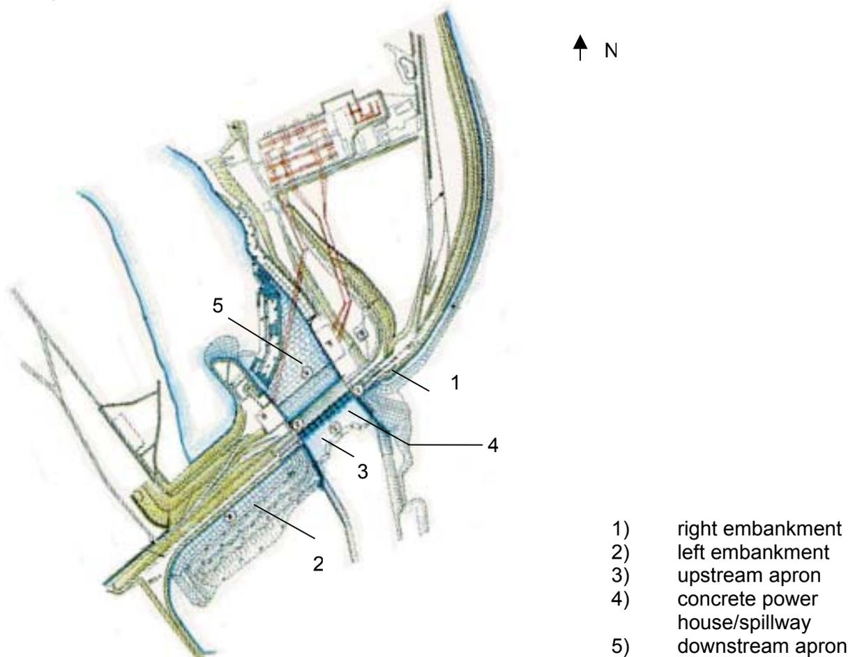
Figure 3: Plan view of Plavinas dam
