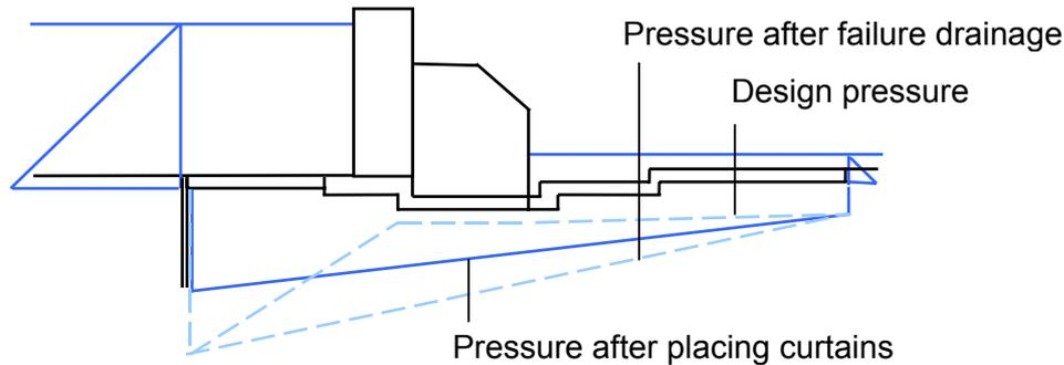
Figure 29: Curtains at the end of the upstream apron
