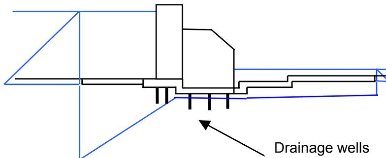
Figure 17: Uplift water pressures due to drainage wells under power house
