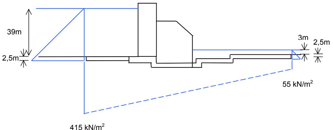
Figure 15: Uplift pressure at the end of the aprons
