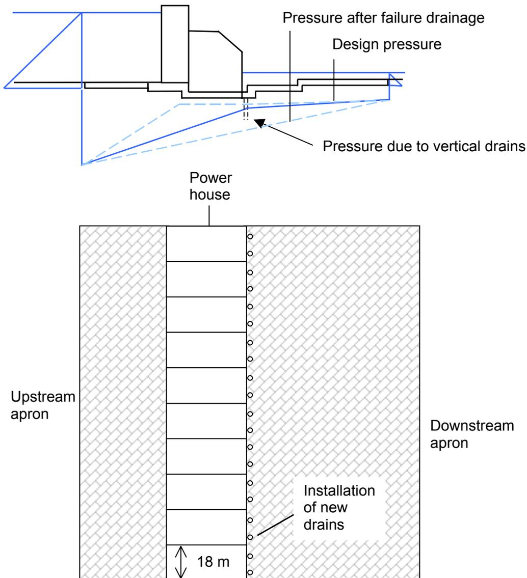
Figure 34: Location new drains in downstream apron
