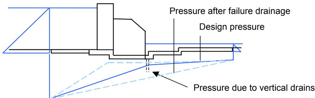
Figure 32: New drains near the power house
