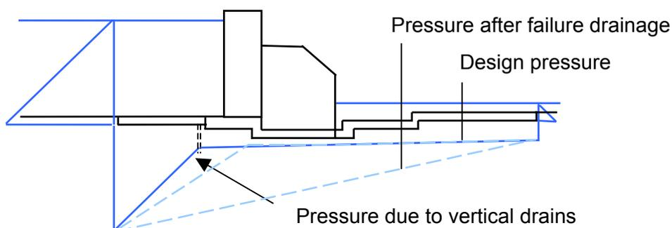
Figure 31: New drains in the upstream apron
