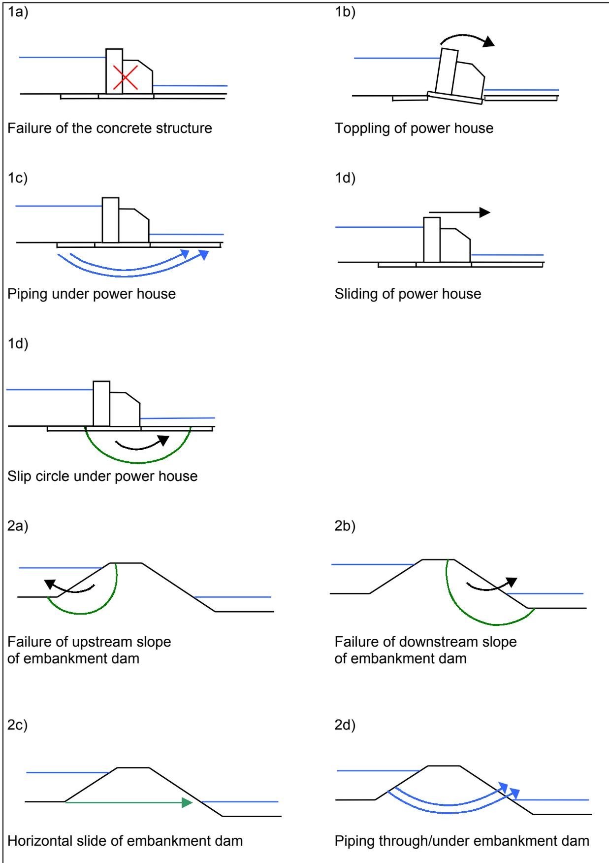
Figure 6: Failure modes for embankment dam and power house structures
