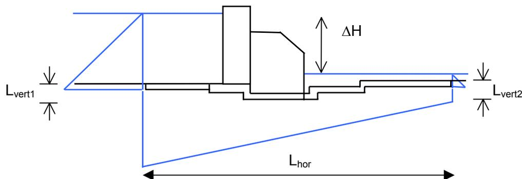
Figure 16: Shape of uplift water pressure distribution under the power house without drainage wells
