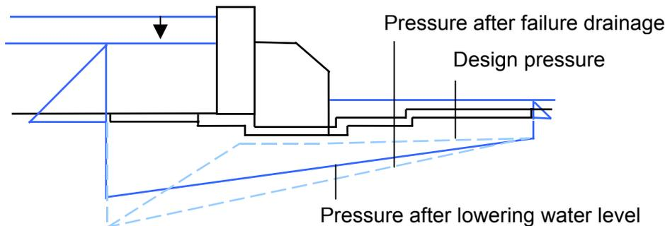
Figure 30: Lowering of reservoir level
