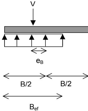
Figure 23: Effective width foundation slab
