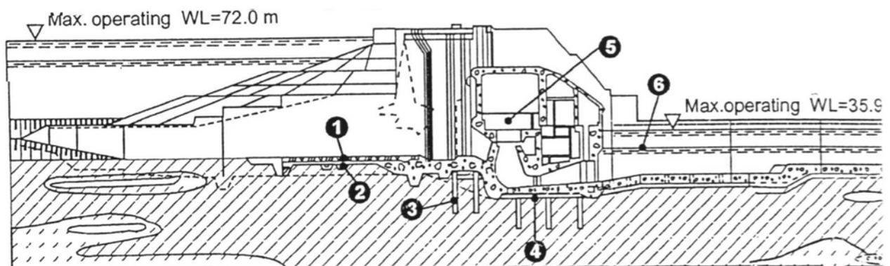
Figure 5: Cross section of Plavinas dam including embankment dam and drainage system
