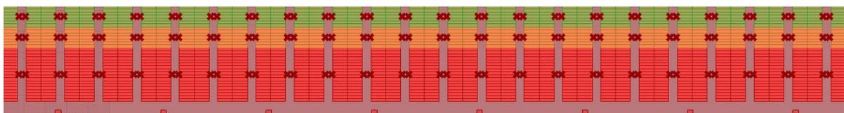
Figure C.23: The generated layout for the scenario "Equally distributed doors over the width of the warehouse when the number of aisles is 22".
