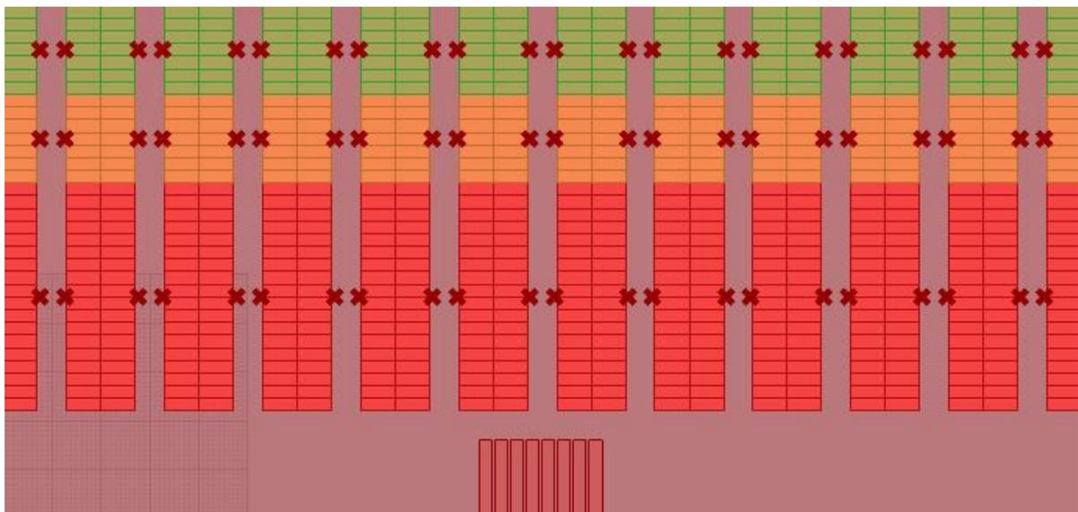
Figure C.13: The generated layout for the scenario "Using double fork FLT's for the transportation task and an ATLS for the loading task".
