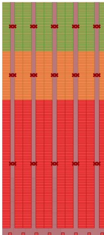
Figure C.22: The generated layout for the scenario "Equally distributed doors over the width of the warehouse when the number of aisles is 5".
