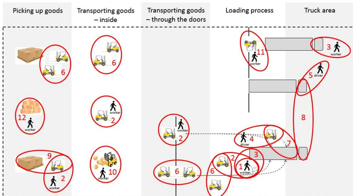
Figure 2.2: A schematic overview of the hazards possibly causing a top three type of accident.
