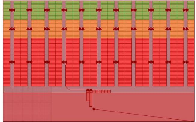
**Fig. 7:** The movements of trucks, truck drivers, transporters and workers are visualised by a dark red line. In this example, a truck arrival and the movement of a transporter between the warehouse and the truck can be seen.
