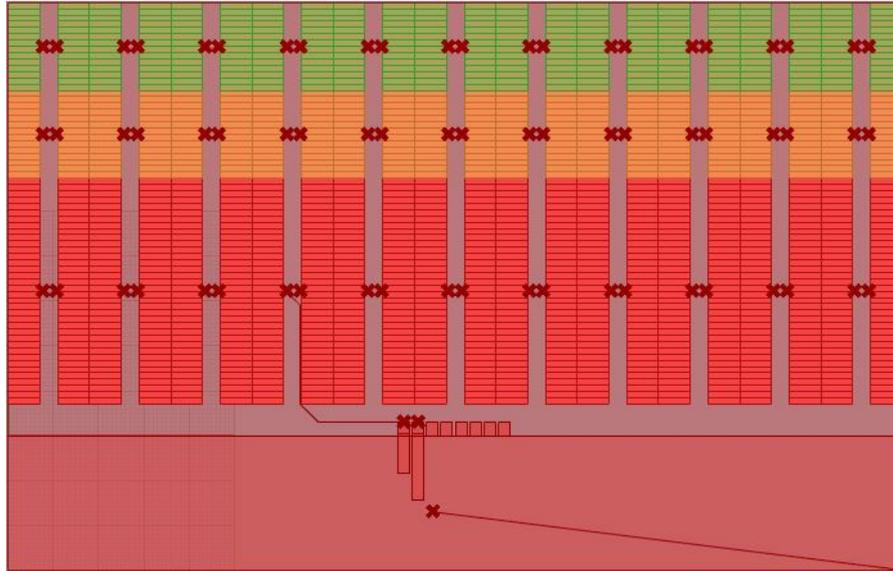
Figure 4.5: The movements of trucks, truck drivers, transporters and workers are visualised by a dark red line. In this example, a truck arrival and the movement of a transporter between the warehouse and the truck can be seen.
