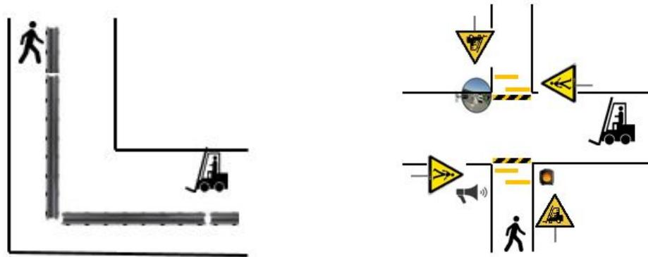
(a) Schematic presentation of the use of a barrier. (b) Schematic presentation of the use of a gate.
