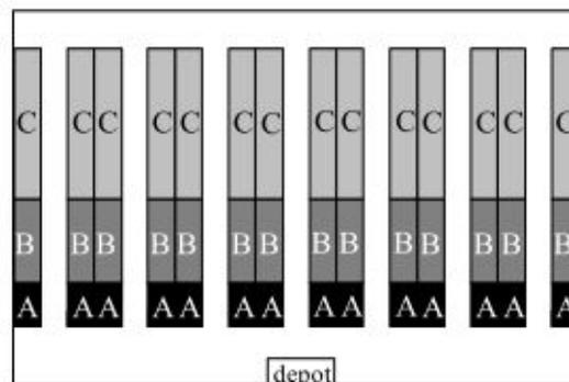
Figure 3.4: A common way to implement class-based storage, retrieved from [Koster et al., 2007]. The products with the highest demand, the A-products, are located close to the loading points. At the moment the truck arrives, these goods can be loaded into the truck quickly.
