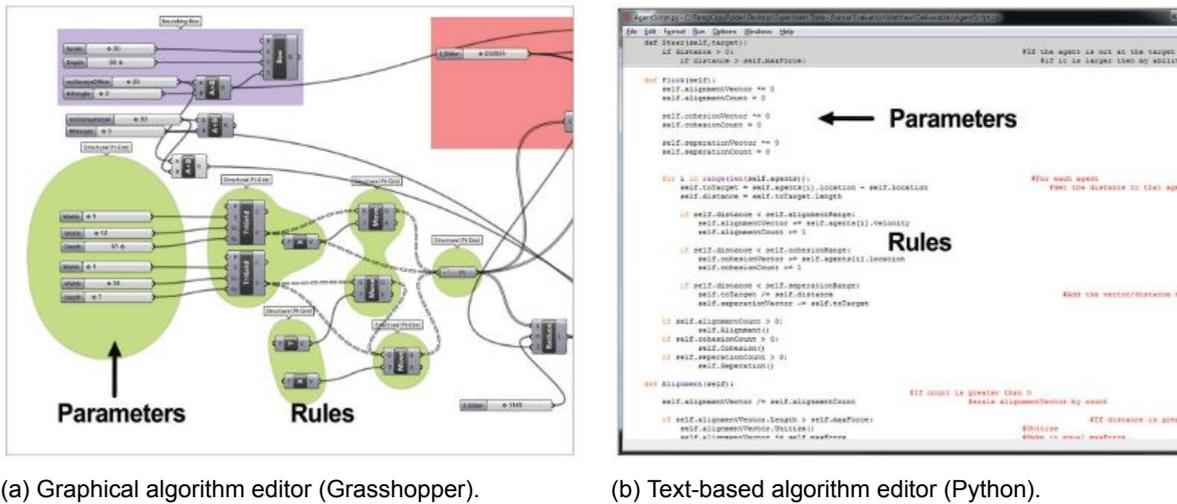
Figure 3.6: Examples of parameters and rules in two different parametric design environments, retrieved from [Lee et al., 2014].
