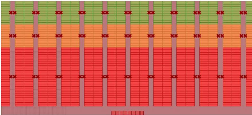
Figure C.4: The generated layout for the scenario "Directly from warehouse - Medium brewery (6 million hL/year)".
