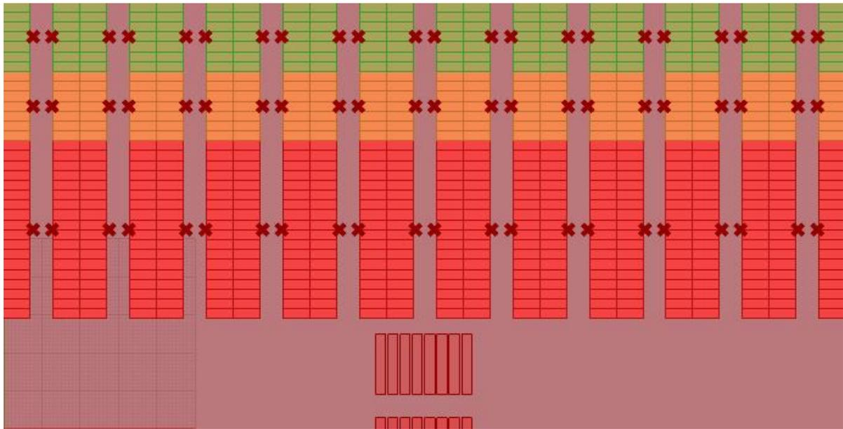
Figure C.12: The generated layout for the scenario "Using double fork FLT's for the transportation task and single LGV's for the loading task".
