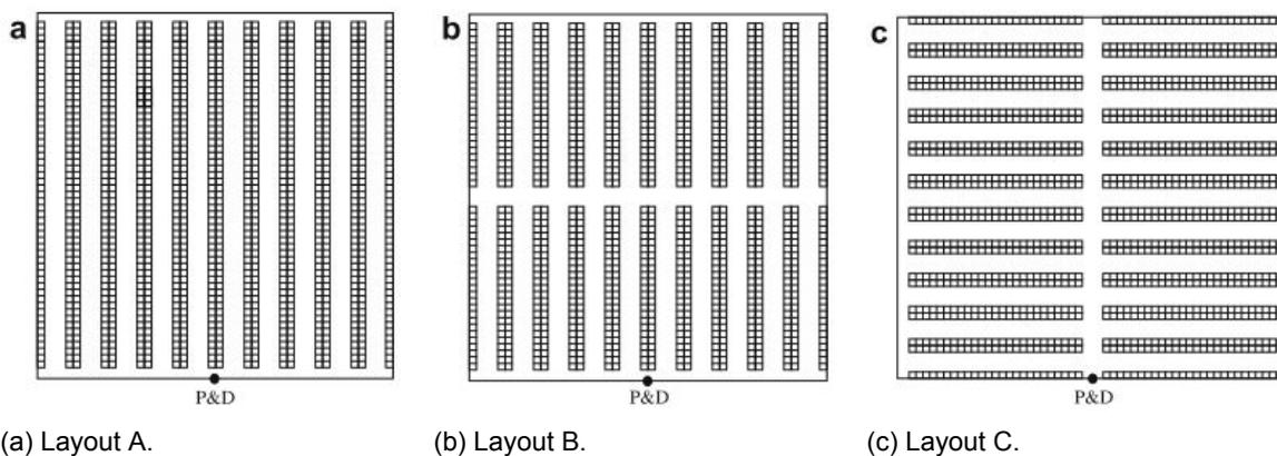
Figure B.1: Three possible warehouse aisle layouts, retrieved from [Pohl et al., 2009].
