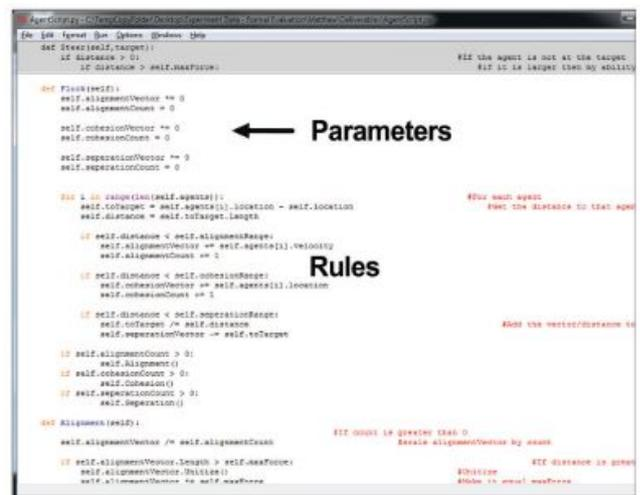
Fig. 3: Examples of parameters and rules in a text-based algorithm editor (Python), retrieved from [Lee et al., 2014].
