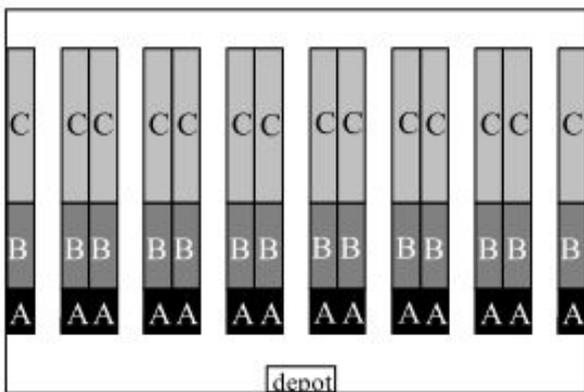
**Fig. 5:** A common way to implement class-based storage, retrieved from [Koster et al., 2007]. The products with the highest demand, the A-products, are located closest to the loading points. At the moment the truck arrives, these goods can be loaded into the truck quickly.
