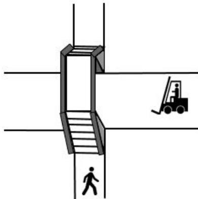
Figure 2.6: A crossing on a different level eliminates the chance of a collision between a worker and an FLT.
