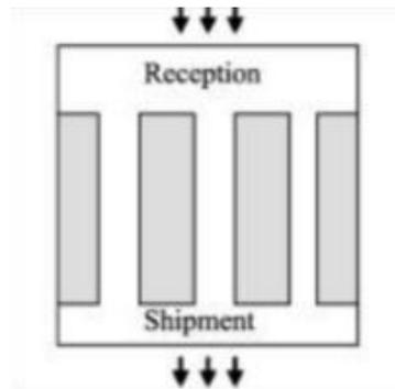
Figure 3.3: Schematic representation of the flow-through configuration, where goods enter the warehouse from one side and are shipped from the other side, retrieved from [Huertas et al., 2007].
