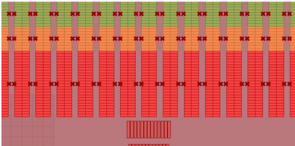
Figure C.9: The generated layout for the scenario "Using pre-staging - Large brewery (11 million hL/year)".
