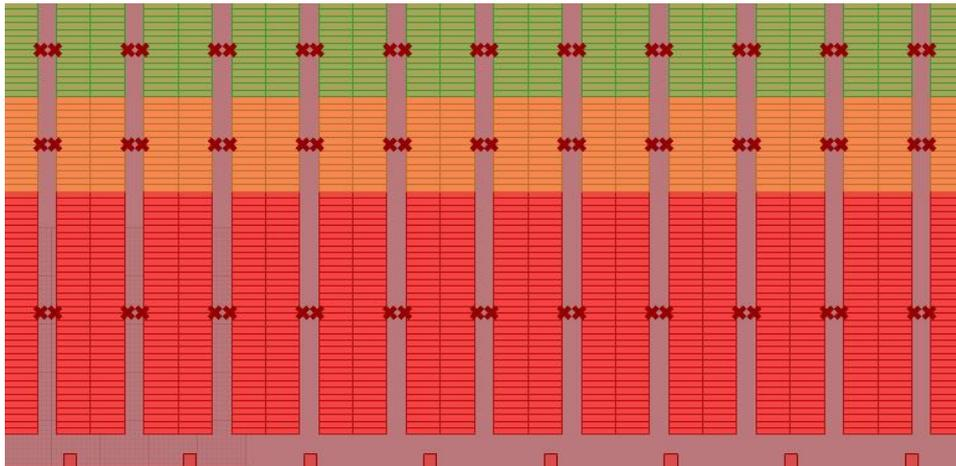
Figure C.21: The generated layout for the scenario "Equally distributed doors over the width of the warehouse when the number of aisles is 11".
