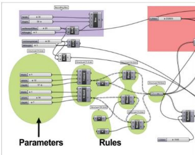
Fig. 2: Examples of parameters and rules in a graphical algorithm editor (Grasshopper), retrieved from [Lee et al., 2014].
