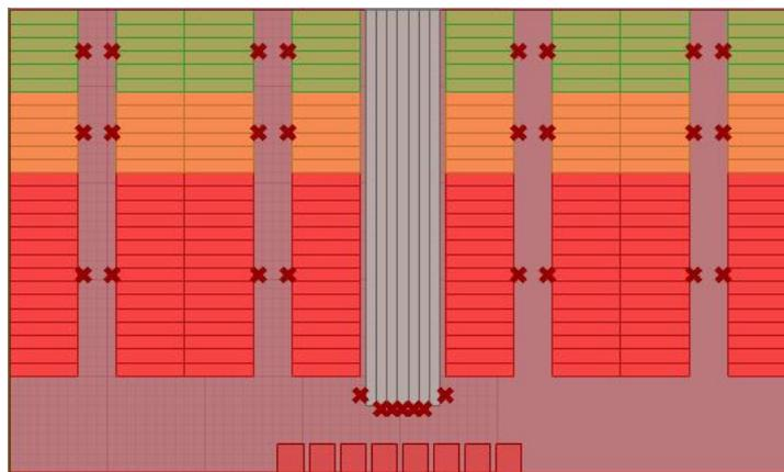
Figure 4.3: Visualisation of the generated layout by the model for the picking process using cross-docking.
