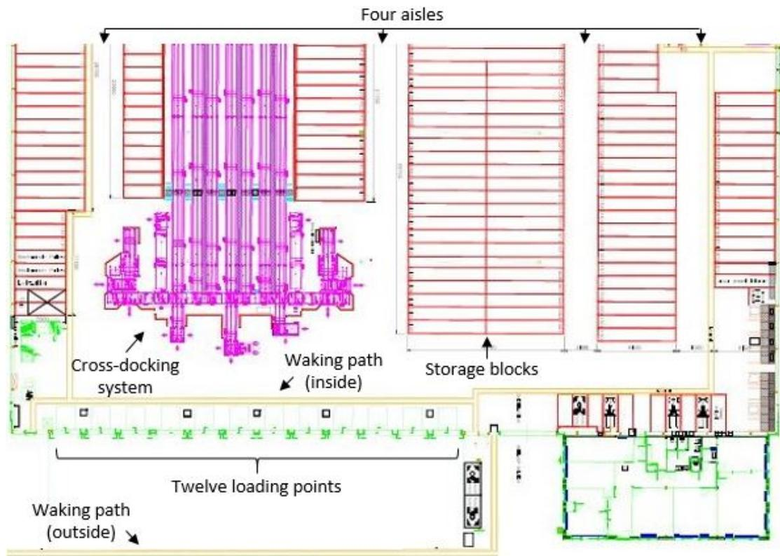
Figure 5.1: Actual floor plan of the warehouse loading area of the brewery in Den Bosch.
