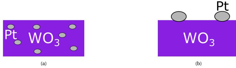
Figure 2.1: Two different ways to combine the catalyst Pt with the  $\text{WO}_3$ ; (a) Pt inside the  $\text{WO}_3$  and (b) Pt on top of the  $\text{WO}_3$ .
