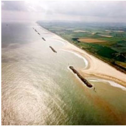
Figure 17: Tombolo Formation Due to Interference with Currents (Bell 2009)
