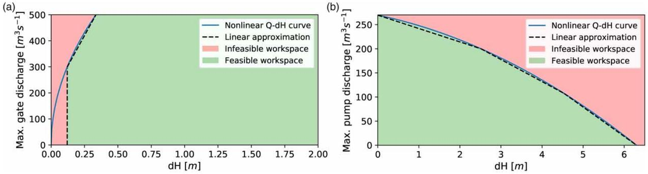
**Figure 4** | Feasible (green) and infeasible (red) region for the discharge from (a) undershot gates and the (b) pumping station in IJmuiden. Please refer to the online version of this paper to see this figure in colour: <http://dx.doi.org/10.2166/hydro.2022.018>.
