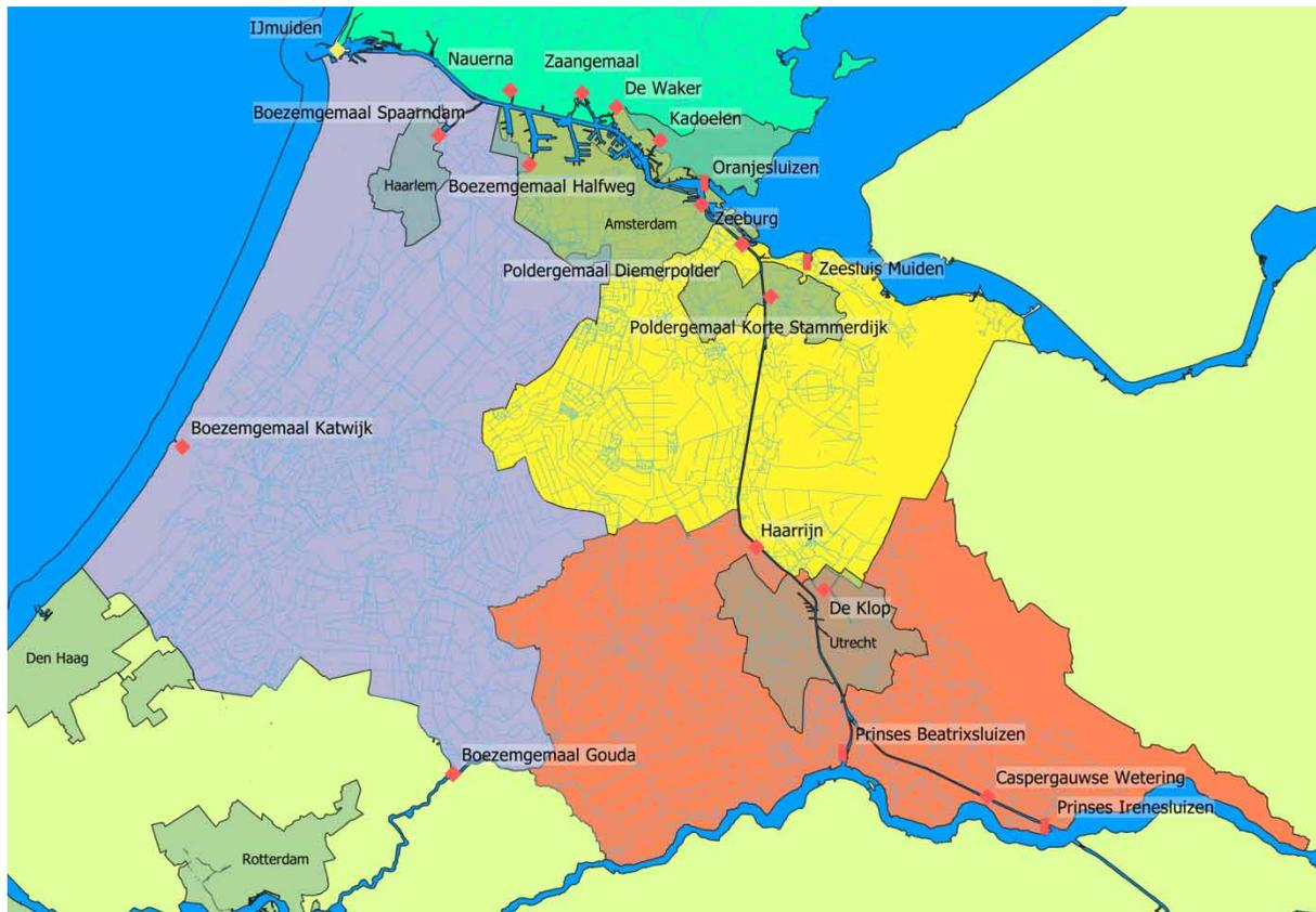
**Figure 3** | The Netherlands, Noordzeekanaal–Amsterdam–Rijnkanaal. The water management area of different local water authorities are shown by color. Inflow and outflow locations of the NZK–ARK are indicated with arrows. Please refer to the online version of this paper to see this figure in colour: <http://dx.doi.org/10.2166/hydro.2022.018>.
