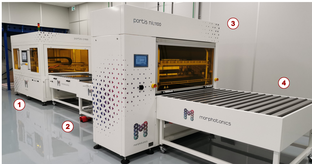
Figure 3.1: The roll-to-plate NIL production line present at Morphotronics, including: (1) the Coater1100, (2) the transport and feed-in table of the NIL1100, (3) the NIL1100 imprint module, and (4) the feed-out table.
