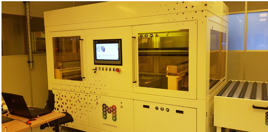
Figure A.1: A photo of the Coater1100, used to perform overlay measurements on Gen5 substrates.
