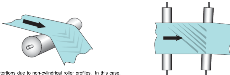
(b) Web distortions due to misalignment in rollers, resulting in an out-of-plane deformation of the web.
