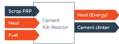
Figure 3-36: Cement co-processing. Image obtained from WindEurope (2020)
