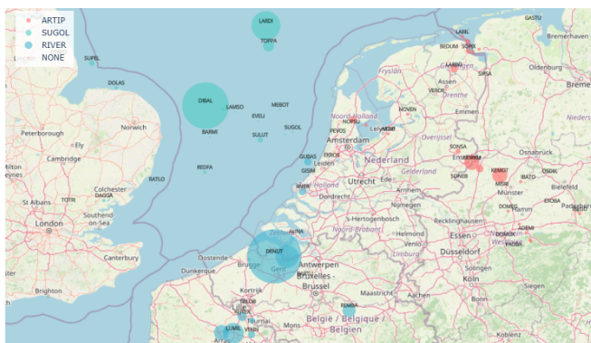
Fig. 10. Bubblemap Indicating Level-Off Location with the Size of the Bubble Indicating the Total Level-Off Duration at that Location
