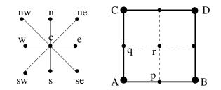
Figure 4: Left: Nine point stencil with numbering, Right: Coarse grid cell and four fine cells (Coarse grid indices by capital and fine grid indices by lower case letters).
