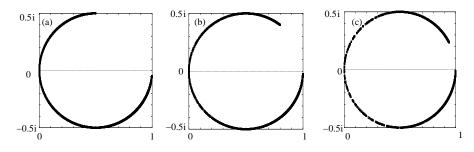
Figure 2: Spectral pictures of  $A_h M_h^{-1}$  for k = 100, h = 1/160 and  $\alpha = 0$ ; a)  $(\beta_1, \beta_2) = (1, 1)$ , b)  $(\beta_1, \beta_2) = (1, 0.5)$ , c)  $(\beta_1, \beta_2) = (1, 0.3)$ .
