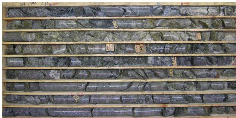
Figure 62 - Corebox with drill core intersecting the crushed zone
