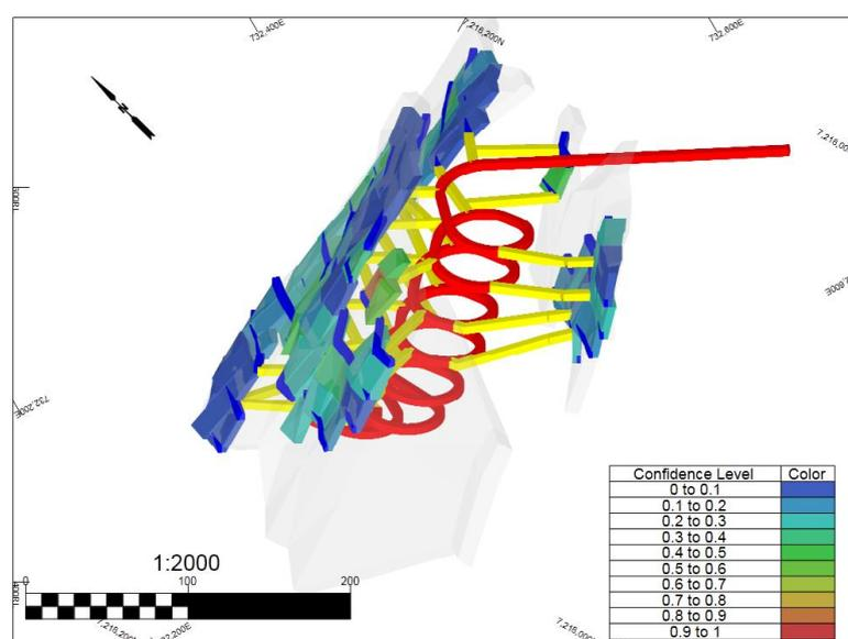
Figure 102 - Directional Estimated Model based stope designs and infrastructure (Au cut-off: 1.8 g/t).
