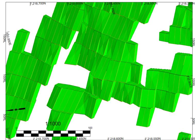
Figure 66 - Framework Optimization example (best scenario @ 1.8 g/t cut-off).
