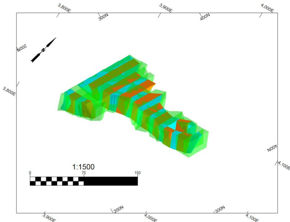
Figure 46 - Stope Optimizer Solution for the 1257 sublevel using 'loose settings'.
