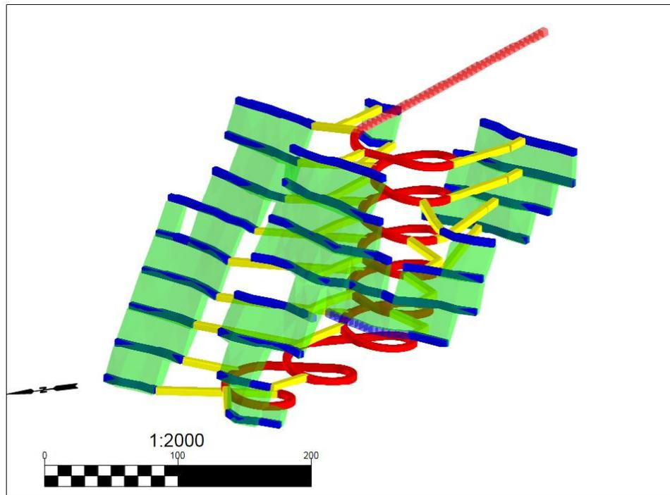
Figure 69 - 1.8 g/t mine design task solids.
