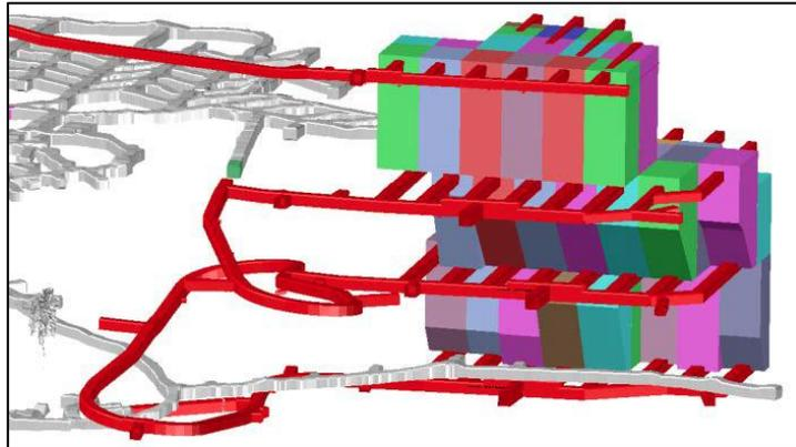
Figure 4 - Transverse stoping in a massive orebody (colours depict different stopes) (Agnico-Eagle Mines Limited, 2012).
