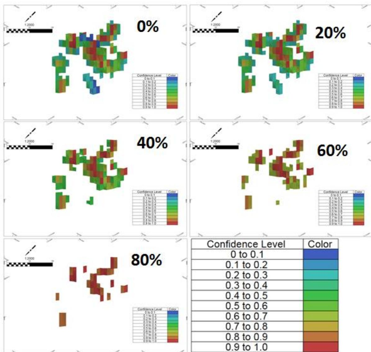
Figure 104 - Optimized Stope Designs at 0-80% minimum confidence level.
