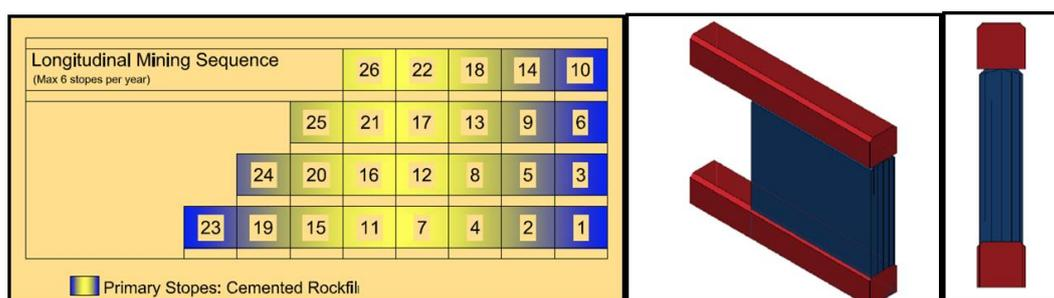
Figure 5 - Longitudinal Stoping in a retreat type sequence (Agnico-Eagle Mines Limited, 2011).
