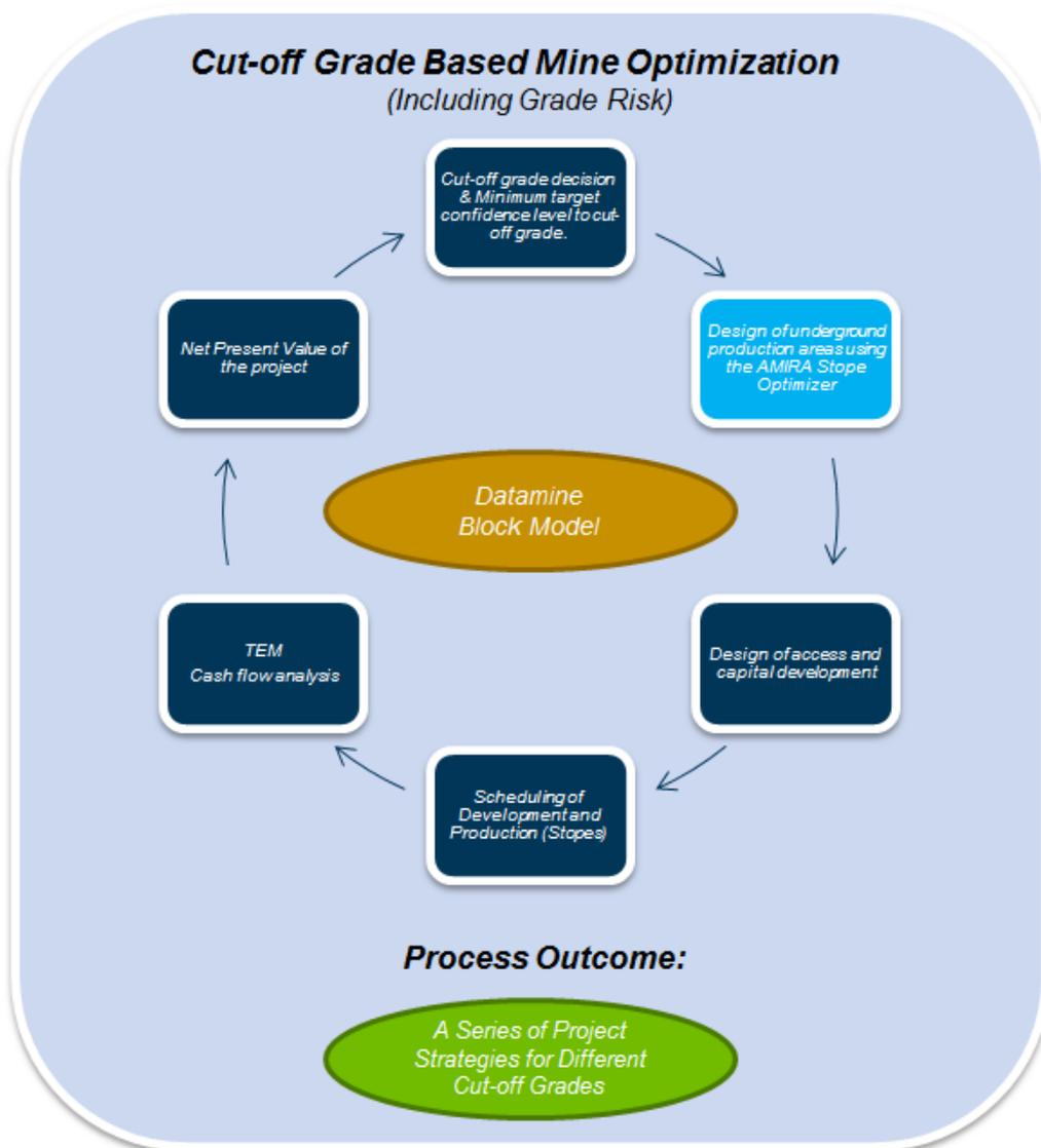
Figure 1 - Cut-off grade based mine optimization (including grade risk).
