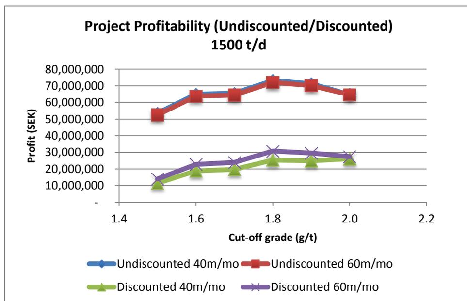
Figure 77 - Base Case Scenario Undiscounted & Discounted Cashflow vs. Cut-off grade - 1500tpd.
