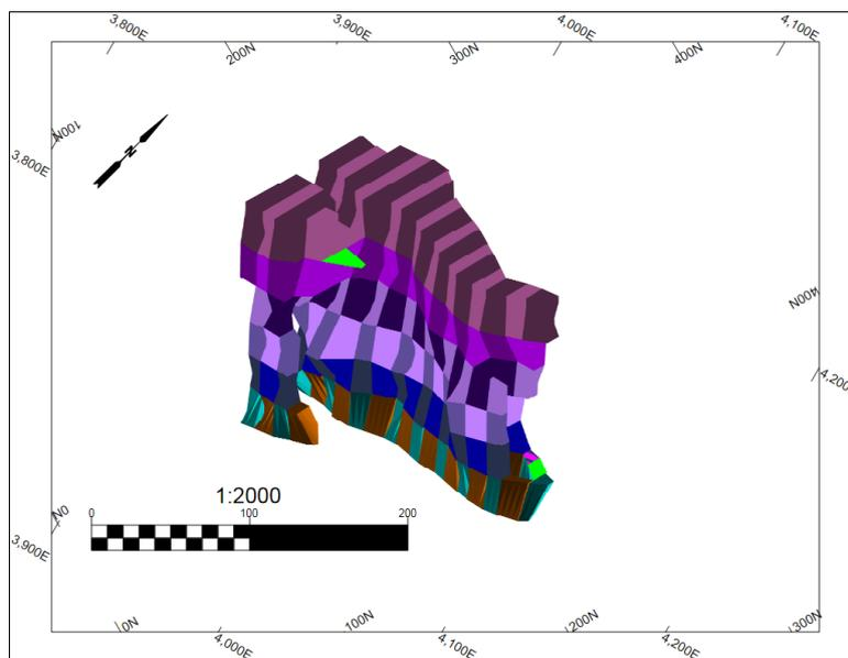
Figure 44 - 2013 Stope Designs for the Lappberget 1250 level.
