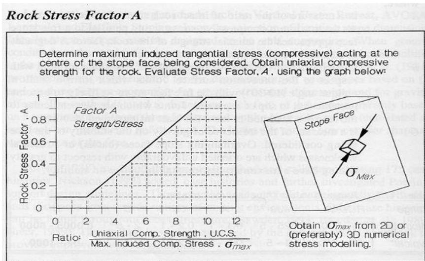
Figure 2.17.1: Rock Stress Factor A (Potvin 1988) for Stability Graph analysis
