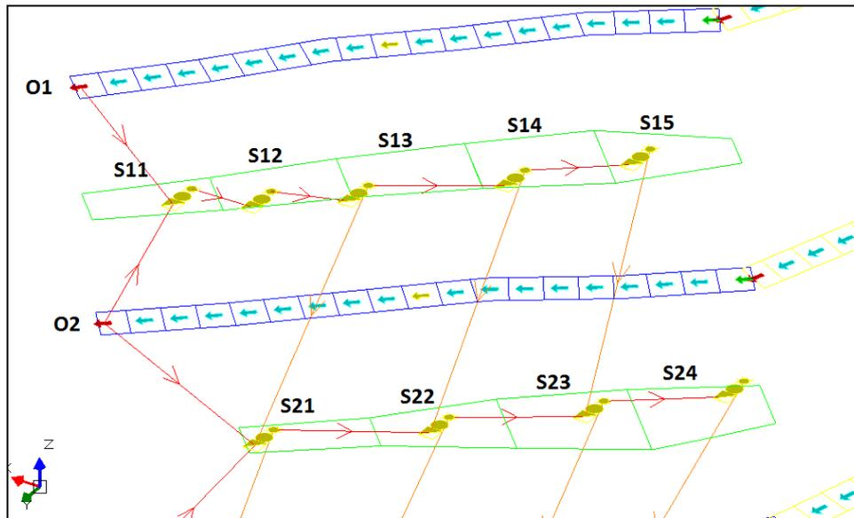
Figure 70 - Lateral & Vertical dependencies (arrows indicating progression direction)
