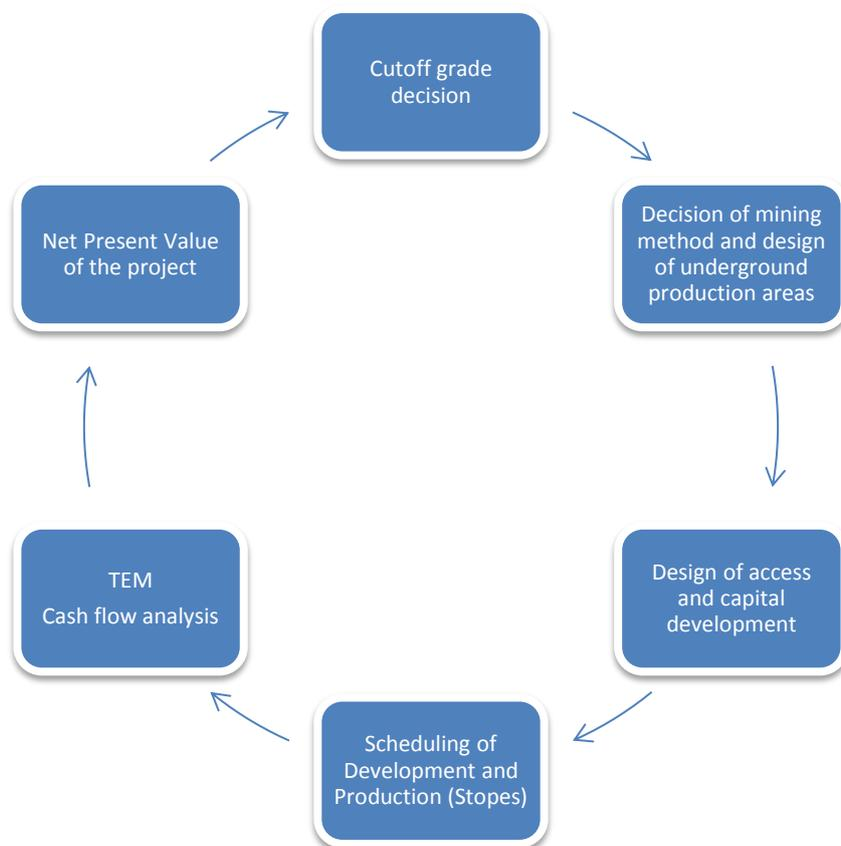
Figure 16 - A typical approach to underground mine planning.
