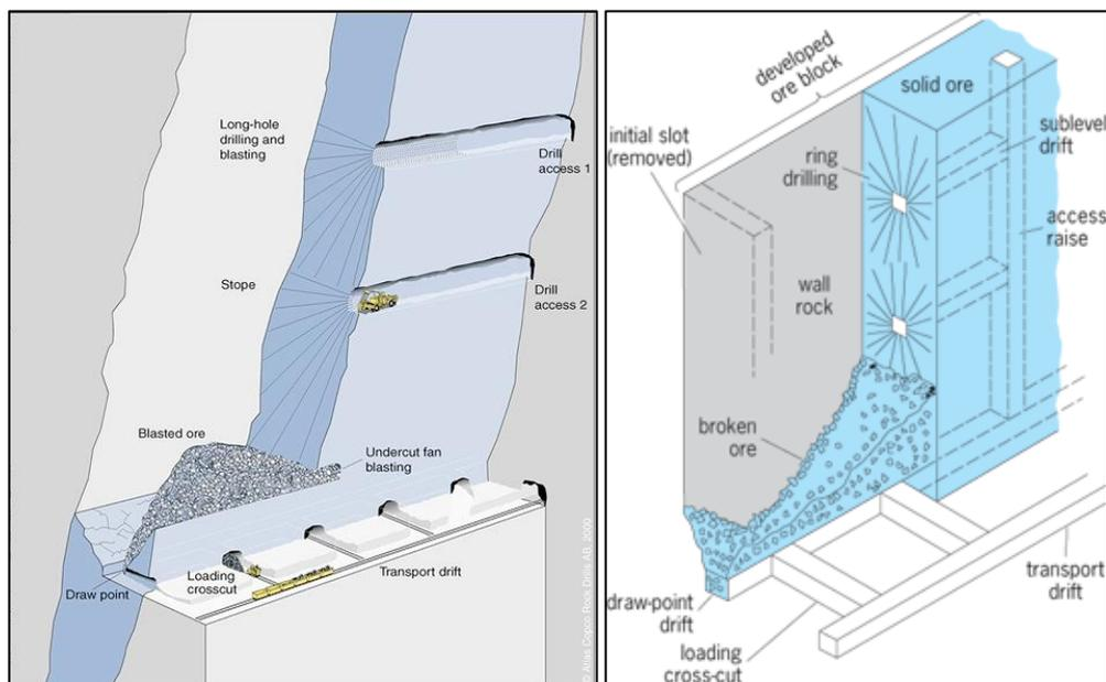
Figure 2 - Sublevel Stoping (tunnelbuilder ltd for Atlas Copco Rock Drills AB, 2007).
