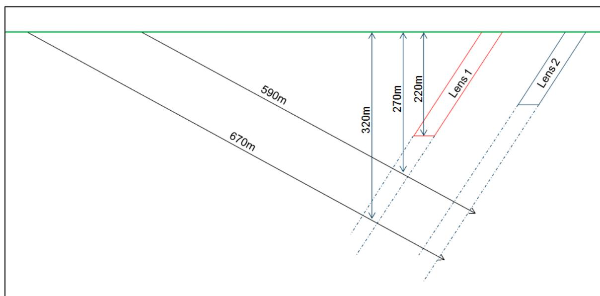
Figure 109 - Schematic representation of proposed drill holes.
