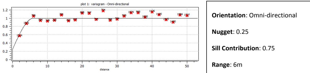
Figure 86 - Omni-directional variogram for grade estimation/simulation.
