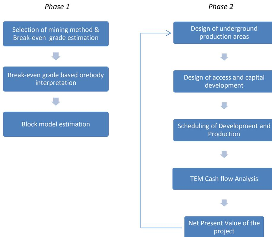
Figure 17 - The Mine Optimization Approach at Boliden
