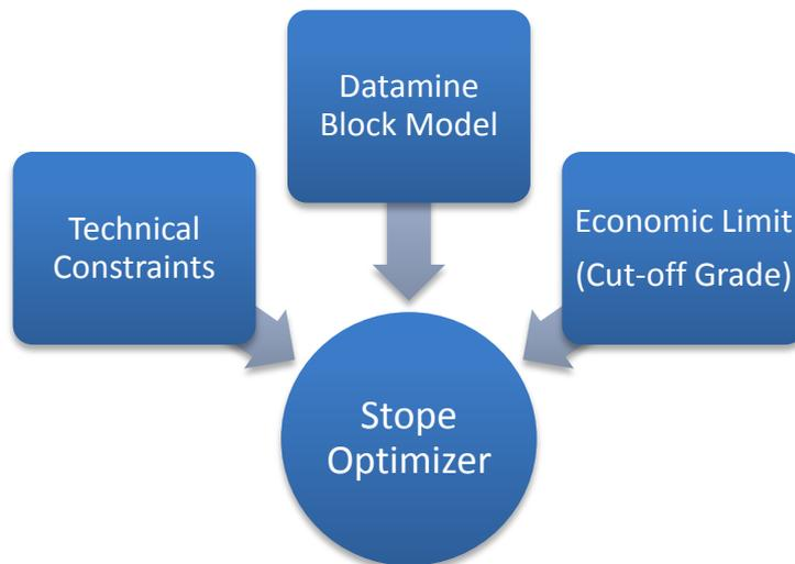
Figure 23 - Inputs into the AMIRA Stope Optimizer.
