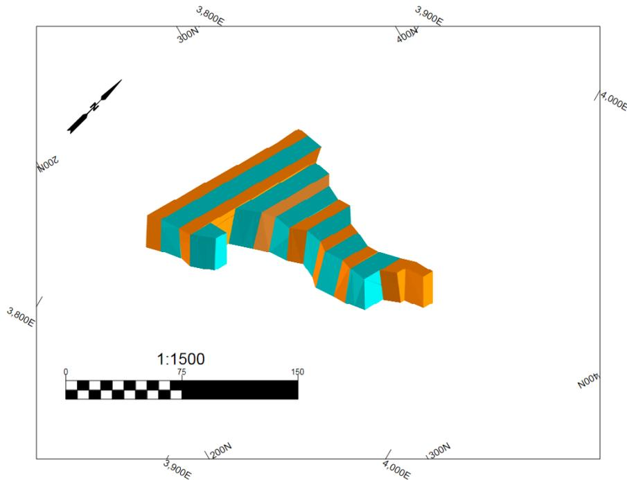
Figure 50 - Final Stope design for the Lappberget 1257 sublevel.
