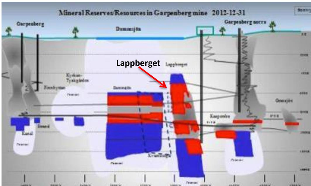
Figure 42 - Garpenberg Mine and Orebody overview (Reserves and Resources shown in Red and Blue respectively).
