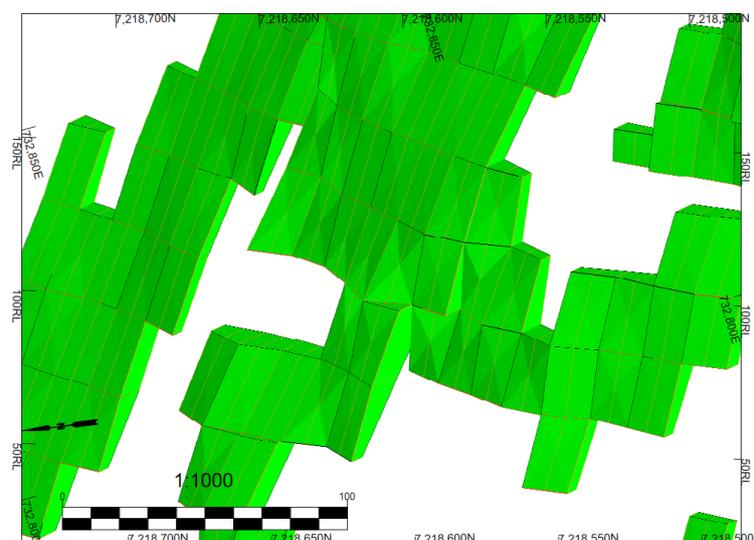
Figure 67 - Optimized Stopes after 'stope smoothing' (best scenario @ 1.8 g/t cut-off).
