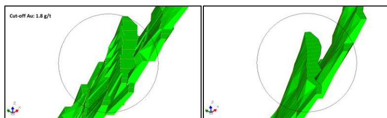
Figure 28 – Optimization output without and with Stope Smoothing.
