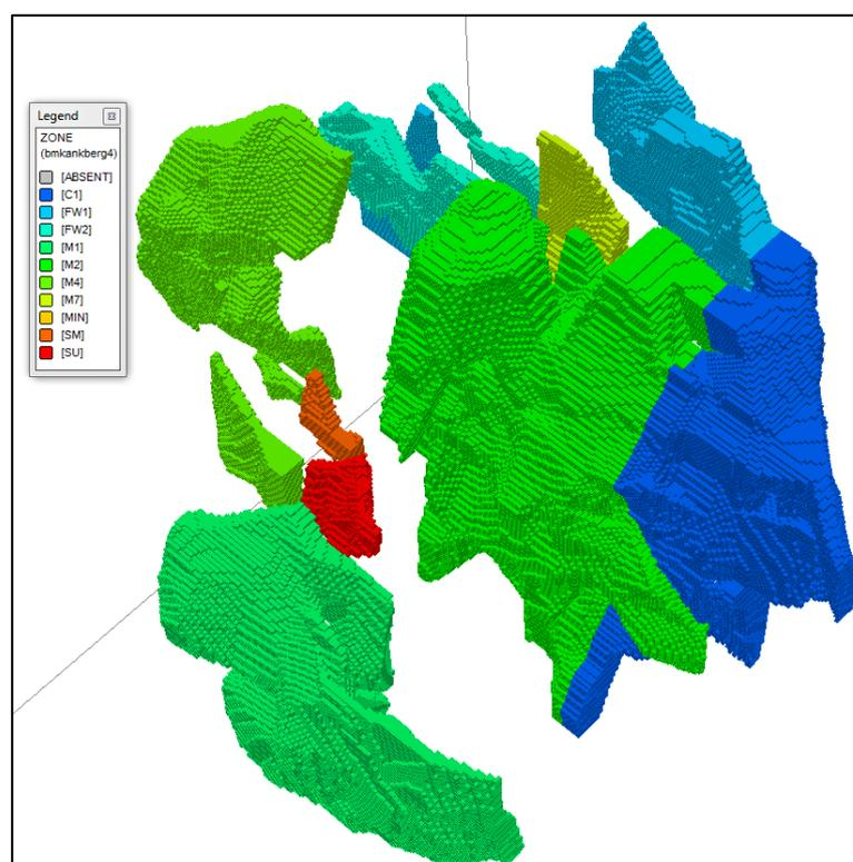
Figure 55 - Kankberg ore zones (Boliden Mineral AB, 2012).
