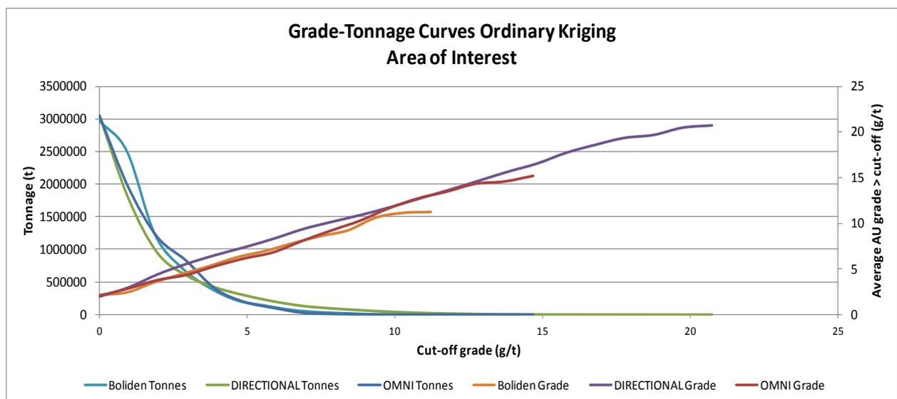
Figure 88 - Grade Tonnage Curve comparison between 3 estimation methods.
