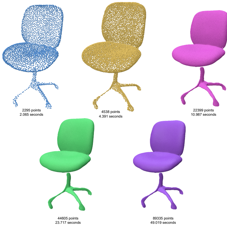
Figure 21: Chair resampled at various sizes using SOLT, along with corresponding sampling times. The results demonstrate that SOLT maintains consistent efficiency and visually coherent output as the sample size increases.
