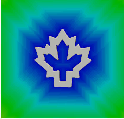
Figure 31: Artificial signed distance function of a maple leaf (computed using our approach).
