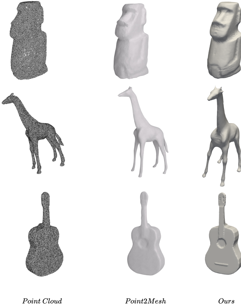
Figure 44: Few point cloud geometries from Point2Mesh [2] along with its output. Our wrap algorithm produces equally smooth results except for a few artifacts created as a result of morphological operators.
