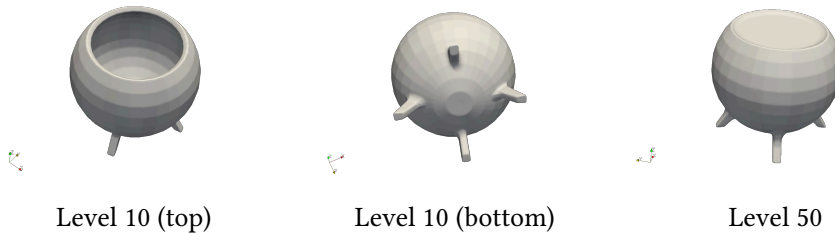
Figure 41: Shrink wrapped geometry for different topological sphere levels.
